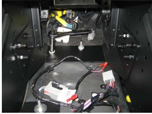
Loosely attach previously removed nuts onto front floor studs. (10mm)
