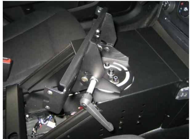
Prior to installation of control heads and accessories, determine desired position and attach Tilt/Swivel and Docking Station bracket.
