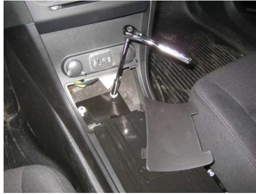
Remove forward O.E.M console plastic cover and remove two (2) nuts from front floor bracket. Nuts to be reused. (10mm)
