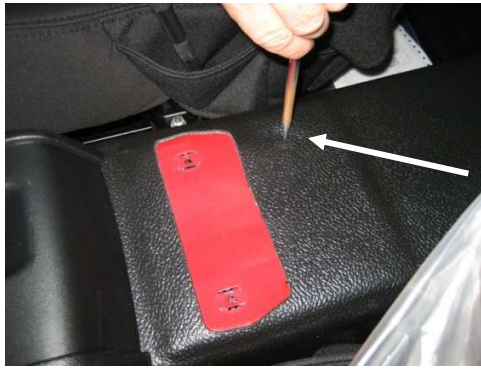
Loosely attach rear of console to existing floor inserts. Inserts located under rubber mat as shown.
