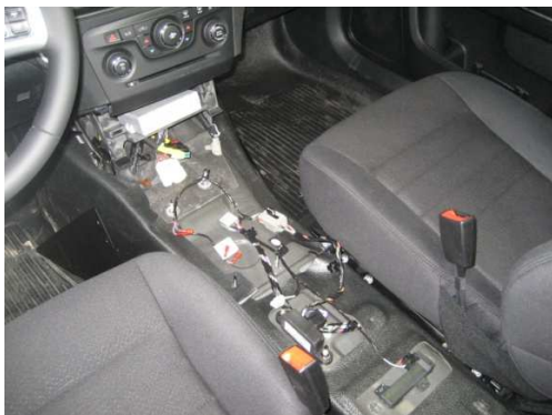
Plug O.E.M. wire harness back onto original connectors.
