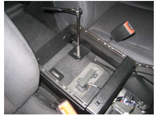
Use OEM screws (if provided) or 1/4 x 3/4 self threading screws (included in hardware kit) to mount rear of console. (7/16 wrench)
