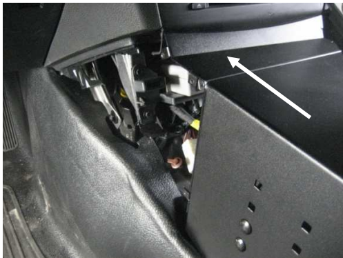
Push Console assembly forward and tighten all floor mount bracket hardware. Run all wiring as needed.
