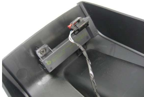
Remove Ignition proximity sensor / antenna from rear underside of O.E.M. console. (Phillips Screwdriver) ** SEE NOTE BELOW **
