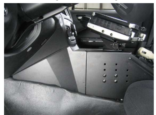
Attach passenger and driver side trim panels on with # 8 x 1/4 Flat Head Screws. (3 screws each panel included with hardware kit)
