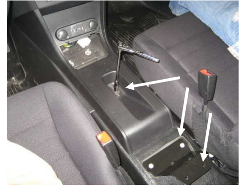
Remove bolts that hold underside of extrusion to rear floor bracket. (7/16 wrench) Remove rear floor bracket bolts and center console bolt. (10mm)
