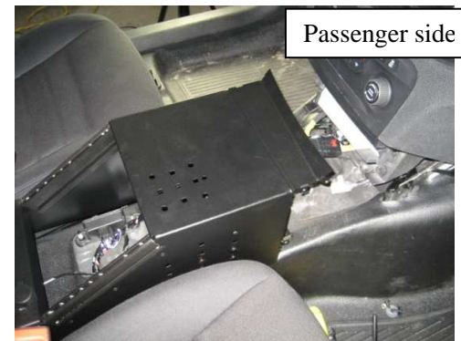
Carefully place console assembly between seats and onto front O.E.M. floor studs.
