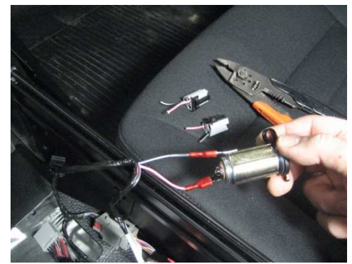
Cut off O.E.M 12 volt socket connectors and attach 1/4 spade connectors on O.E.M. wires. O.E.M. wire will need to be extended for rear socket. If desired, new heavier gauge wires can be installed instead of using O.E.M. wiring.
