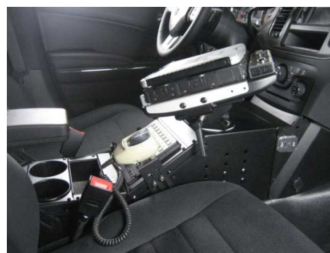
Reconnect under dash "AUX" USB connectors back together. Plug spade connectors onto 12 volt sockets. Positive Pink wire connects to center (silver) spade and Negative Black wire to outboard (gold) spade.
