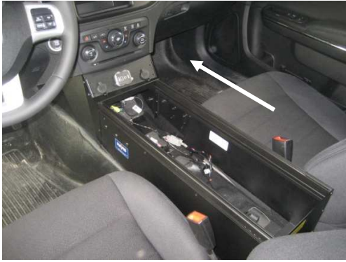
Push Console assembly forward and tighten all floor mount bracket hardware. Run wiring as needed.
