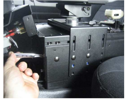
Install Control heads and accessories. If necessary, remove side trim panel for easier computer mount bracket access.
