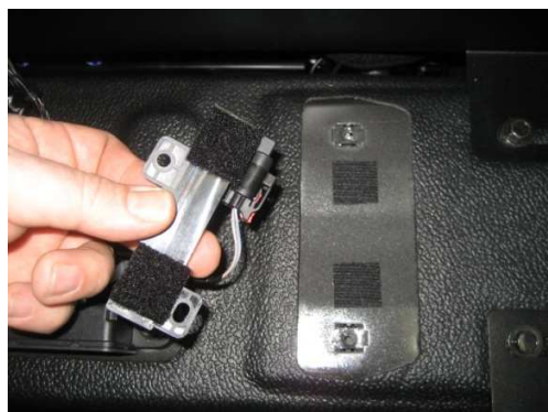
Attach self adhesive Velcro pads onto bottom of Ignition proximity sensor /antenna and to transmission hump. Note: Newer cars may include a bracket with this sensor already relocated. If so, Velcro will not be needed.
