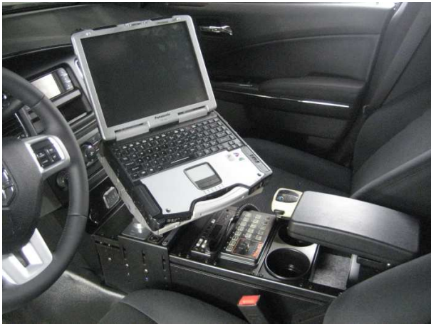
Completed console installation with Laptop / Docking Station (example 1)
