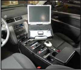
Havis Consoles are manufactured from bent and welded steel for superior durability. They also feature our unique aluminum extruded side rails, which make adding and positioning options and accessories simple while allowing them to remain adjustable. Each console is also designed to work with Havis' mounting options and accessories as well as our docking stations and computer mounts.
