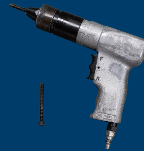
2 Pneumatic Rivnut Gun bolts
