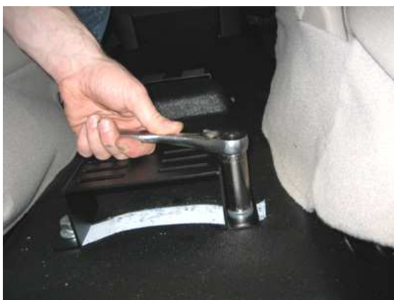
Tighten all floor hardware.
