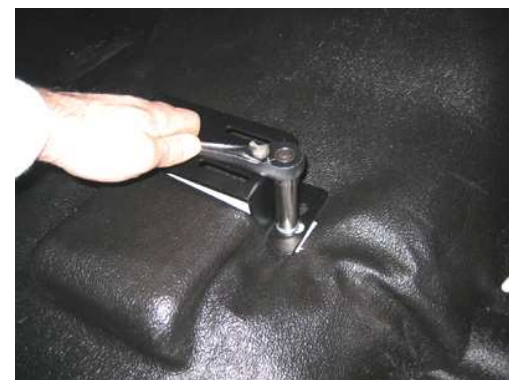
Repeat these steps on the rear holes using the 1/2 x 1" Thread cutting bolts.
