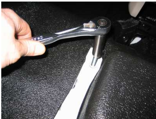
With the floor plugs removed, tap out the (2) forward holes with the 3/8 x 1" Thread cutting screws.
