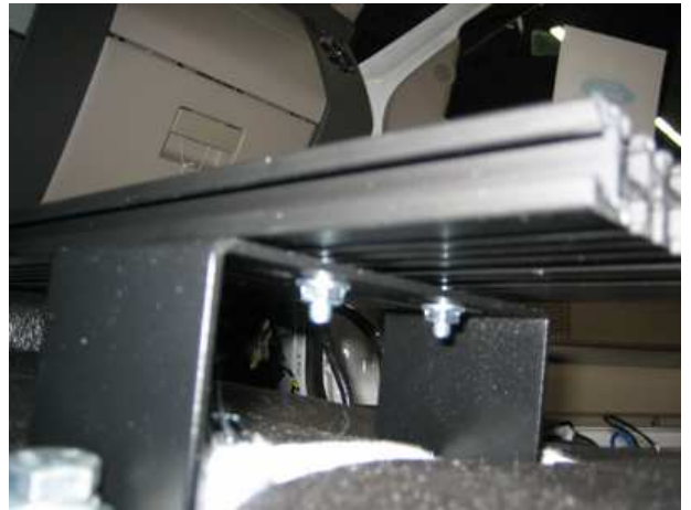
Attach the tunnel to the C-B10's using 1/4" serrated nuts. Adjust Trak to desired position and tighten hardware.
