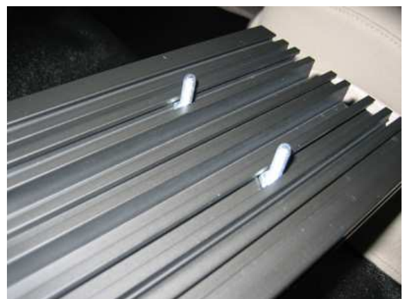
Repeat these steps on the rear holes using the 1/2 x 1" Thread cutting bolts.
