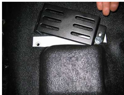
Install the C-B10 mounting brackets using the same 3/8 x 1" screws
