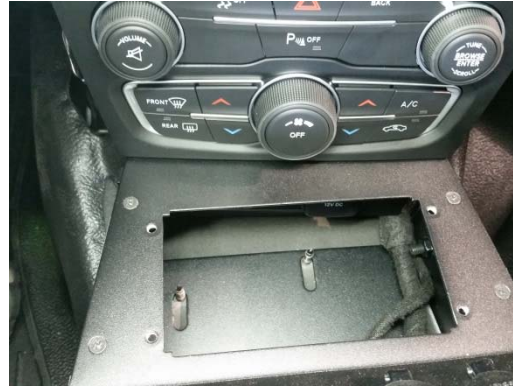
Place console up to dash and remove the accessory pocket. Attach the two (2) supplied M6 flange nuts to the OEM studs.
