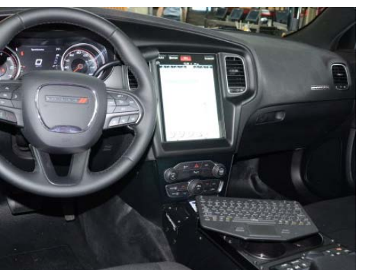
Console housing installation is now complete.
