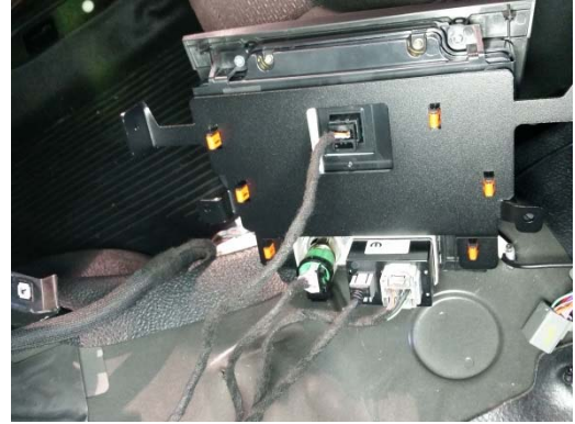
Attach the HVAC support bracket to the OEM control. Make sure all six (6) clips are fully seated in the bracket.
