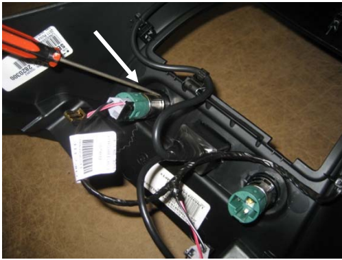
Carefully remove O.E.M. 12 volt sockets and "AUX" socket from OEM plastic panel. Small flat screwdriver can be used to push sockets out.
