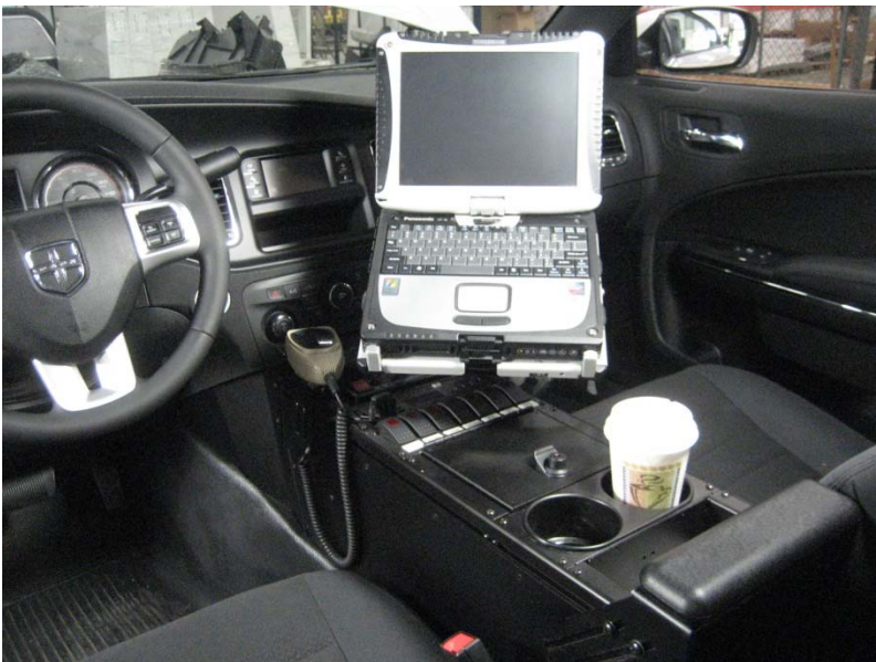
Completed console installation with Laptop / Docking Station
