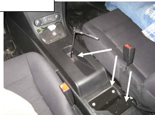
Remove bolts that hold underside of extrusion to rear floor bracket. (7/16 wrench) Remove rear floor bracket bolts and center console bolt. (10mm)
