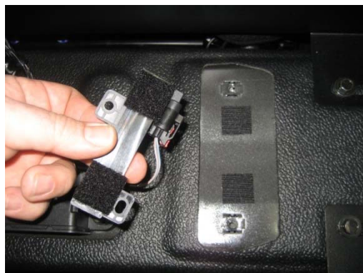
On 2011 Charger, attach Ignition proximity sensor /antenna to transmission hump with Velcro. NOTE: 2012 and newer cars include an O.E.M. bracket with this sensor already relocated. Velcro mounting will not be needed
