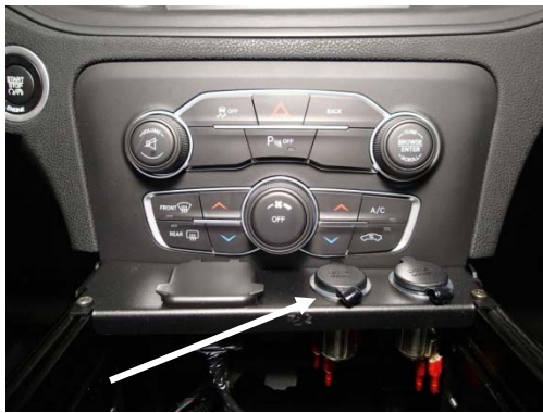
Two (2) aftermarket 12 volt socket kits #C-HK-184 are included with this Charger console. The installer has the option to use either the OEM or Aftermarket 12 volt sockets. (C-HK-181 socket shown installed)
