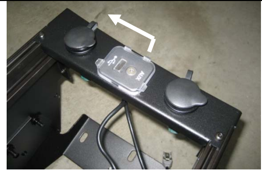
Firmly push in the O.E.M 12 volt sockets and Auxiliary socket assembly into center End Panel Cutout. "AUX" lettering goes to passenger side.
