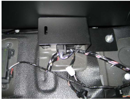
A Cover is provided to guard the O.E.M. Sensor on transmission hump. Attach to existing stud and 6mm nut and washer provided.
