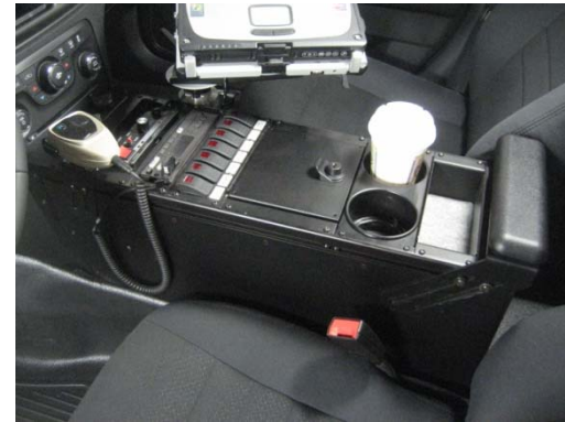
Install Control heads and accessories. If necessary, remove side trim panels for easier wiring access during installation
