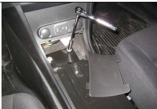
Remove forward O.E.M console plastic cover and remove two (2) nuts from front floor bracket. Nuts to be reused. (10mm)
