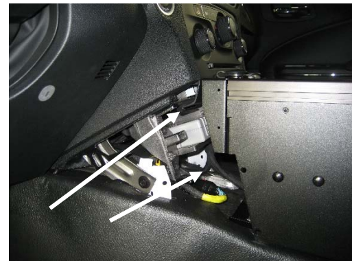
Plug 12 volt sockets and "AUX" USB connectors back together. Note: When placing console onto floor, it is best to leave front bracket attached to console and slide assembly forward into position.
