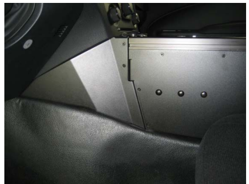
Attach driver side trim panel on with # 8 x 1/4 Flat Head Screws. (included with hardware kit) (Phillips Screwdriver) After console housing is firmly mounted, remove panel as needed to run wires
