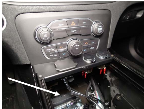
Carefully place console between seats and onto front O.E.M. floor studs. Loosely attach previously removed nuts onto floor studs. (10mm)
