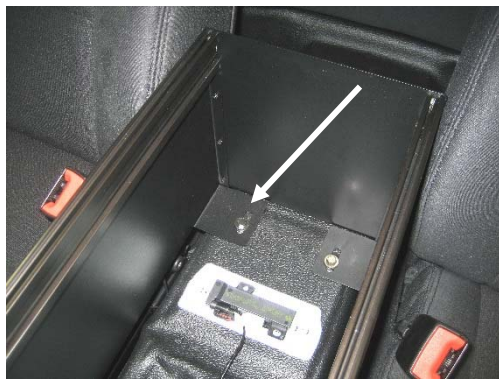
Use 1/4 x 3/4 self threading screws (included in hardware kit) to loosely attach rear of console to existing floor inserts. Inserts located under rubber mat as shown. (7/16 socket)
