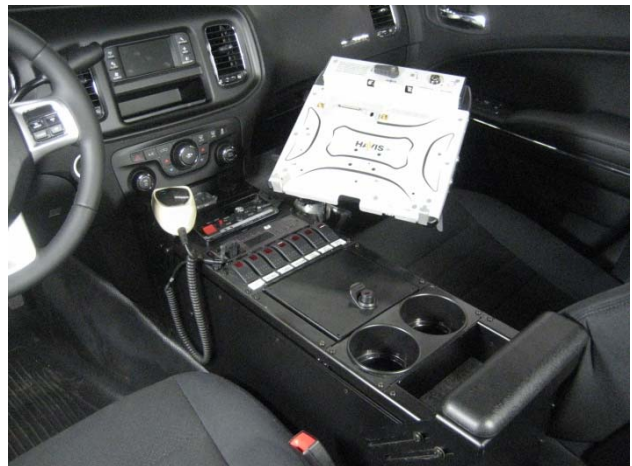
Completed console installation with Docking Station.
