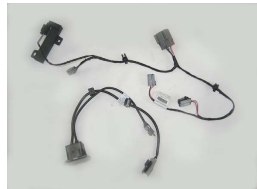
Remove sensor and 12 volt socket wire harness assembly from under side of O.E.M. console. Pop out "AUX" socket from center of O.E.M console.
