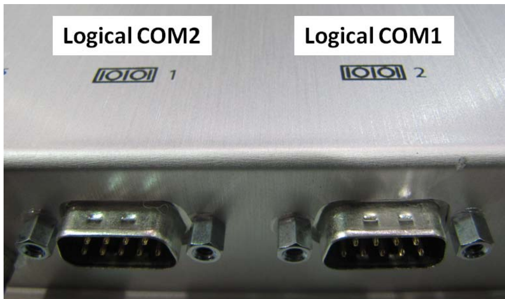
BOTTOM VIEW of DS-PAN-110 Docking Station (Future product will have serial port designations removed)
