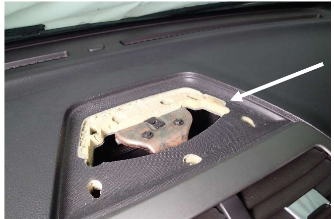
Attach driver side upper support bracket to dash as shown with existing screw. (7mm socket) Torque to 3 Nm (27 lb in)
