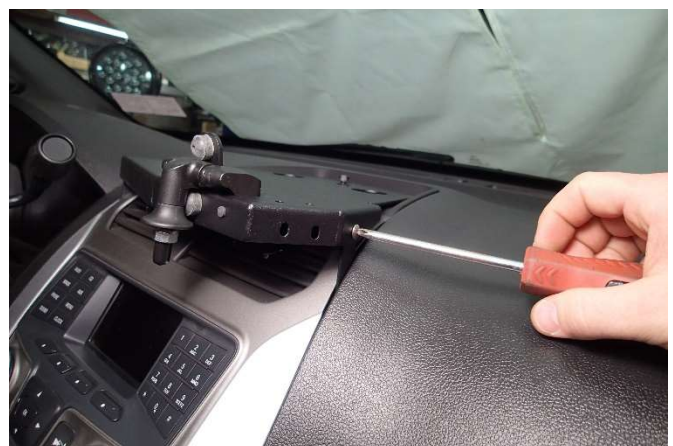
Attach main dash mount bracket to side upper support brackets with 8-32 x .312" Phillips head machine screw and tighten all mounting hardware. (Phillips screwdriver)
