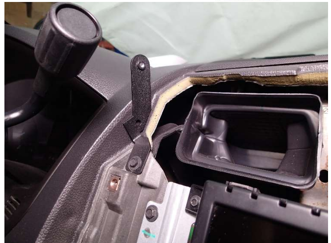
Attach driver side upper support bracket to dash as shown with existing screw. (7mm socket) Torque to 3 Nm (27 lb in)
