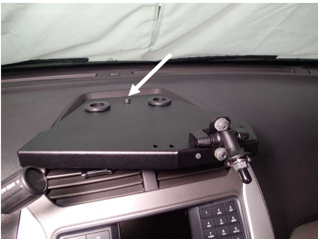
Place the aluminum spacers into pocket on top of OEM trim panel. Place main dash mount bracket on top and attach with M6 x 45mm Hex head bolt. (10mm socket) Torque to 3 Nm (27 lb in)
