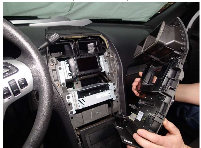
Remove and unplug center instrument panel assembly.
