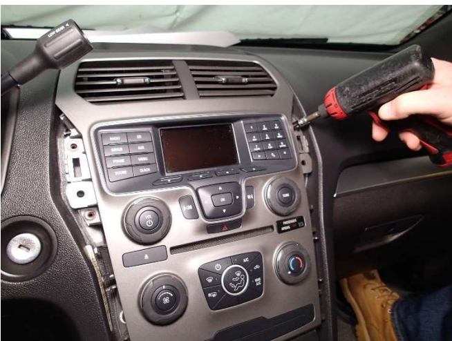
Unscrew center dash assembly. (7mm socket)
