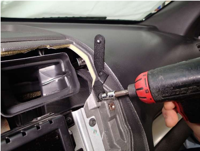
Attach passenger side upper support bracket to dash as shown with existing screw. (7mm socket) Torque to 3 Nm (27 lb in)
