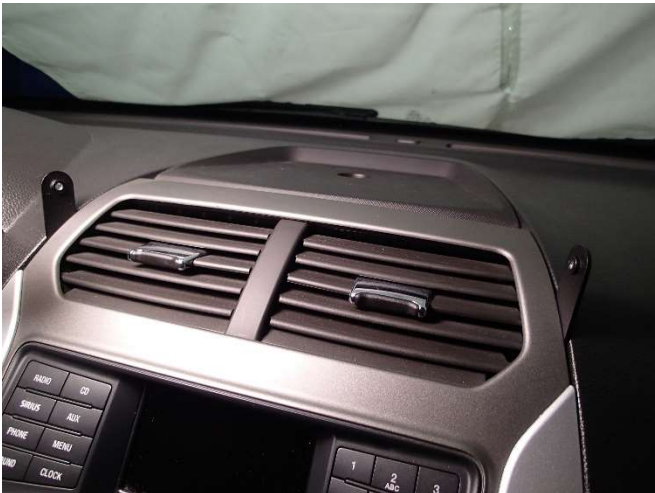
Plug in and remount center instrument panel assembly.
