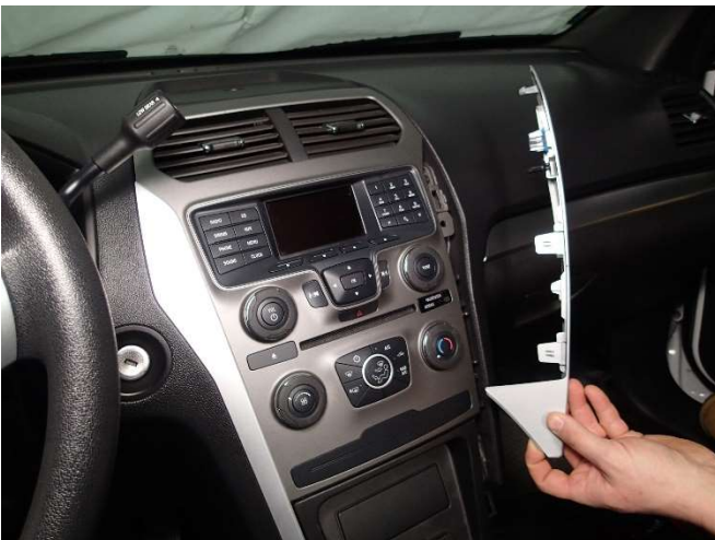
Passenger side trim panel removed.
