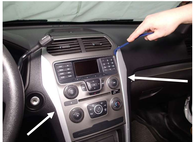
Carefully remove the center dash side trim panels.
