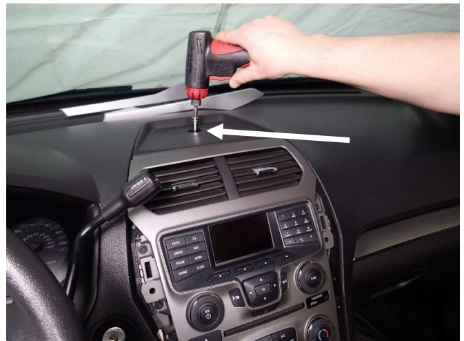
Remove bolt from top center dash panel.
