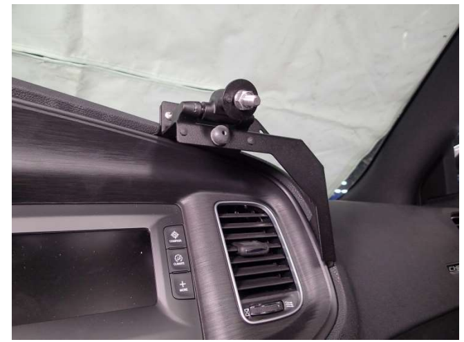
Re-install previously removed frame bracket
