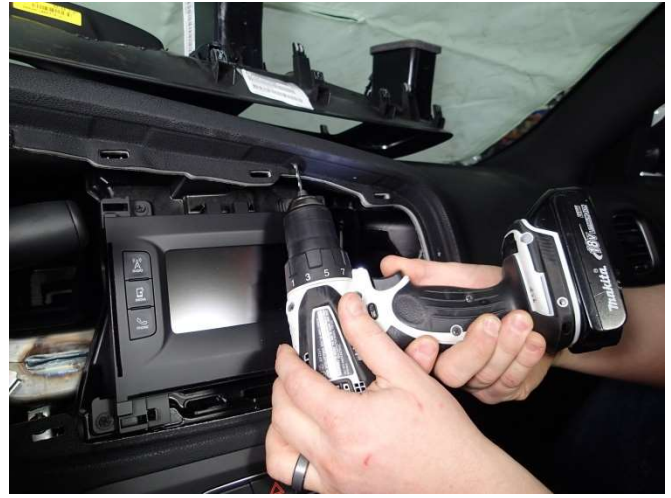
Use 1/8" drill bit and carefully drill your pilot holes.
