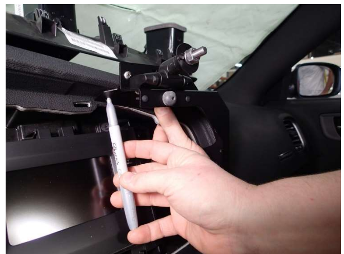
Mark holes to be drilled with a paint marker.
