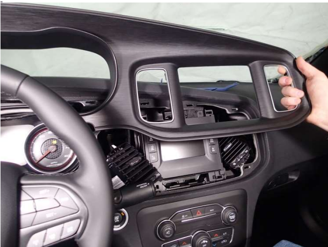
Remove dash bezel. The vents may stay in the dash upon removal.
