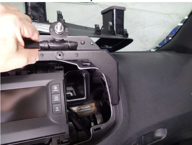
Hold C-DMM-2004 bracket assembly up to inside lip on dash to determine approximate mounting location.
