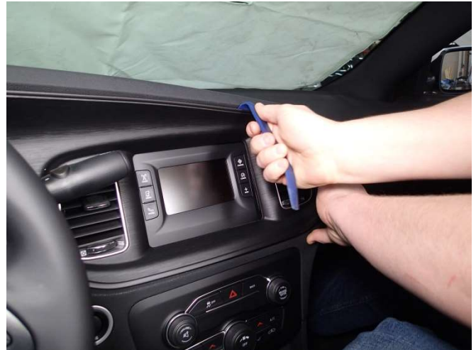
Gently pry along the edges of the dash to release the clips.
