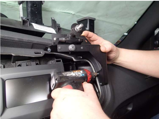
Install the bracket assembly using four (4) 10 x 3/4" Self tapping screws.
