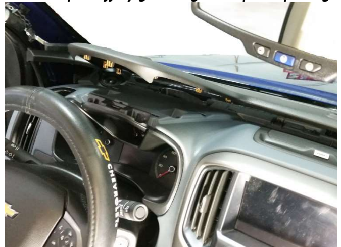
Pry up and remove front top dash trim assembly.
