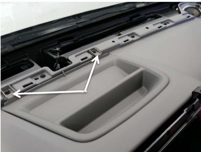
Remove two (2) 7mm head fasteners from upper center tray. Pull tray towards the windshield and remove.
