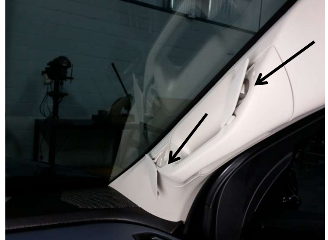
Remove passenger "A" pillar trim by removing two (2) 10mm head bolts located behind covers on grab handle. Driver side will pull off by grabbing the top and pulling down.
