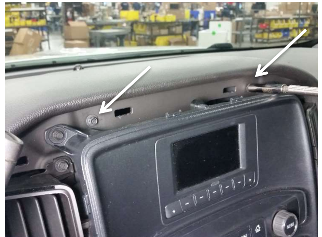
Remove fasteners above radio display (7 mm socket)
