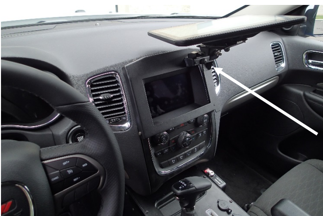
Attach bracket with display to the tilt swivel hinge with M8 hex nut and lock washer. Tighten nut and attach vinyl cap on M8 bolt threads.
