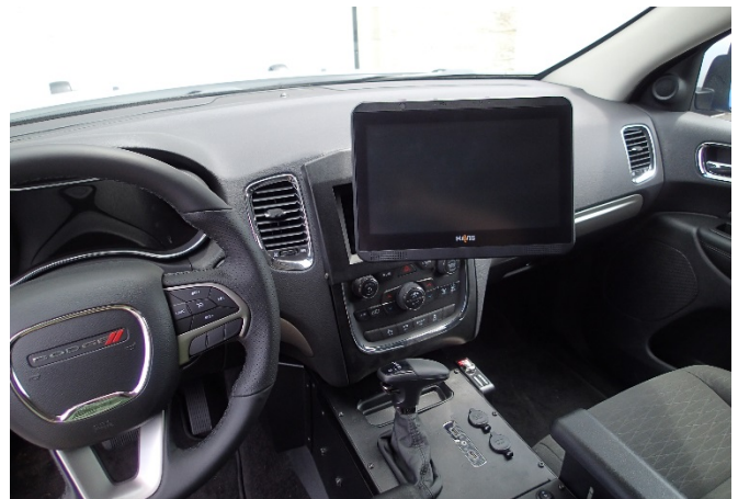
Carefully run and strain relief wiring. Refer to TSD-201 owner's manual for power and computer connection details. Installation is now complete.
