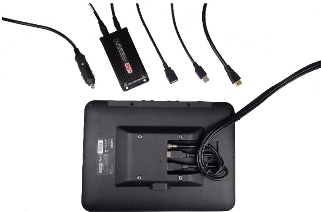
Connect harnesses to the back of the TSD-201 display. It is important to also double wire tie the harnesses to provide sturdy strain relief for the plugs.
