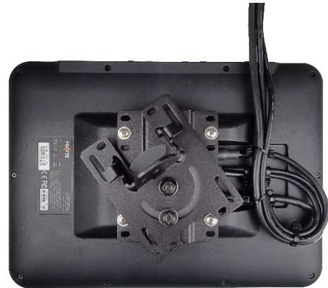
Attach the DMM frame to the lower side brackets using 10-32 x 1/2" screws, flat washers, and Keps nuts.
