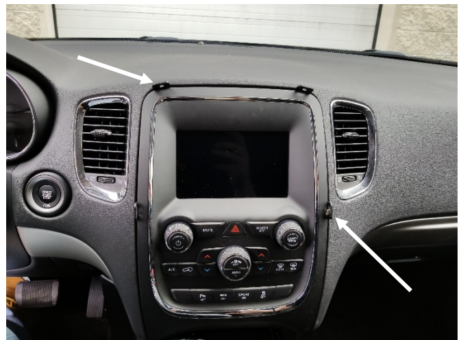
Carefully reinstall trim bezel / panel assembly with four brackets protruding out of gap between bezel and dash.
