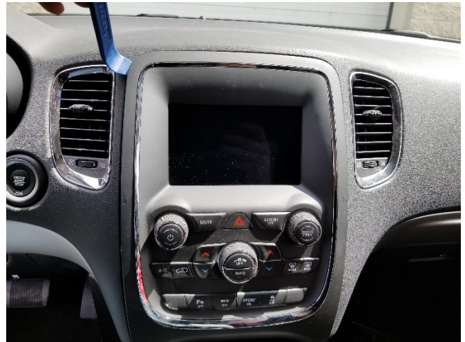
Carefully remove trim bezel / panel assembly using plastic panel tool.
