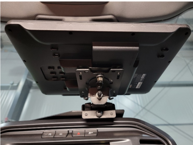
Attach bracket with display to the tilt swivel hinge using M8 hex nut and lock washer. Tighten nut and attach vinyl cap on M8 bolt threads.
