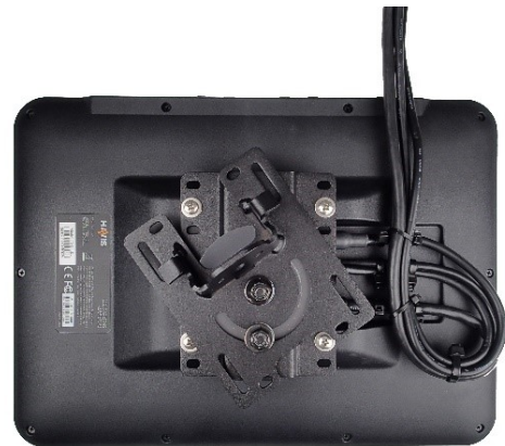
Attach pivot / display mount bracket to display with M4 x 0.7 x 10mm Phillips head machine screws, lock washers and flat washers. Display mount hardware is included with TSD-201 hardware kit.
