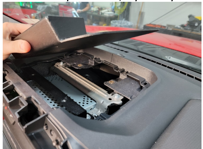
Place C-DMM-2023 frame onto dash.
