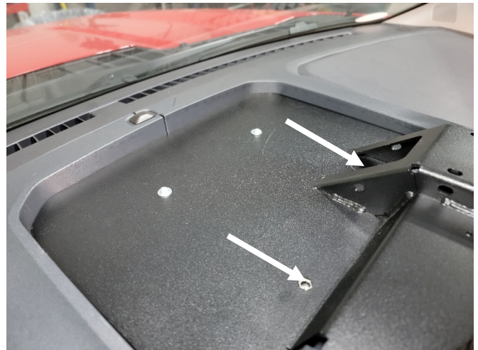
Attach rear section of DMM tray to dash using (2) 10-32 x 3/4" Machine screws and flat washers
