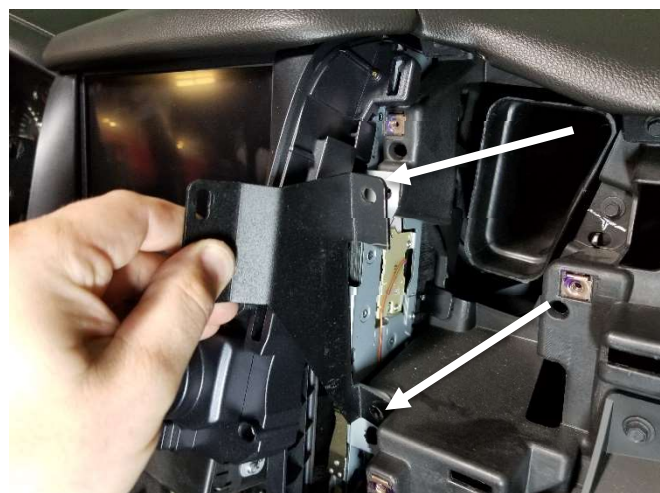
Remove two (2) screws on each side next to the OEM screen. Install side support brackets using OEM hardware.
