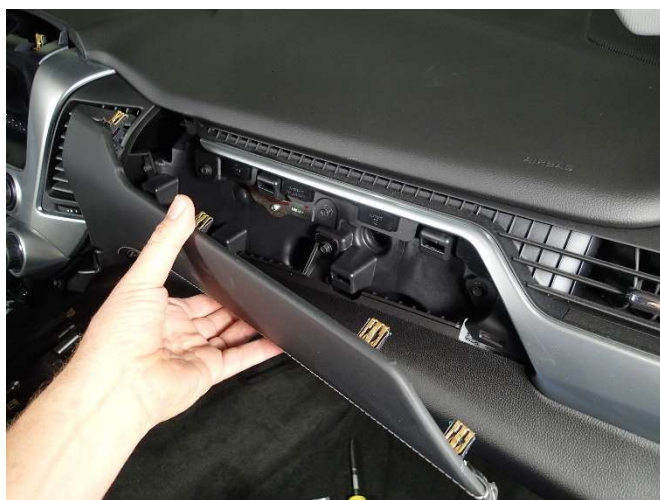
Insert a flat blade panel removal tool and remove the panel above the glove box.
