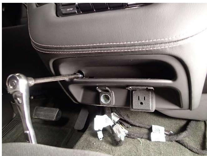
Remove rubber cover in lower accessory pocket to gain access and remove two (2) lower dash panel screws. (7mm socket)
