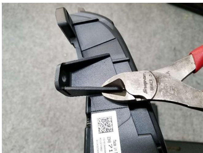
On the 2017 and older Tahoe, (2) plastic tabs will need to be trimmed. This can be done with a simple snip from a pair of diagonal cut pliers
