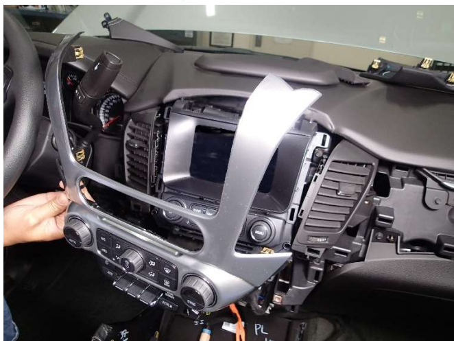
Carefully remove (unsnap) center trim bezel around touch screen and climate controls
