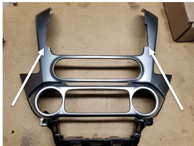
Carefully notch trim bezel accordingly and reinstall back into dash. Re-install all vents and dash trim. File or Dremel tool works well for notching plastic.
