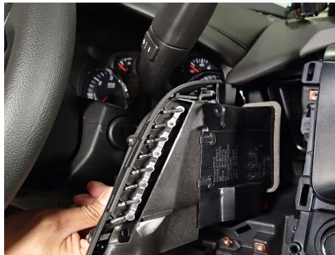
Remove three (3) screws from the vent housing and remove the housing. Repeat for passenger side. (7mm socket)
