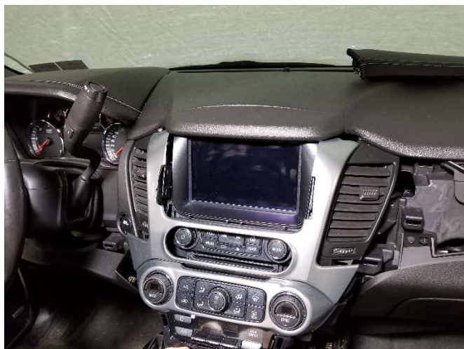
Loosely place the center trim bezel up to the dash and mark the plastic area around the upper side brackets to be notched.
