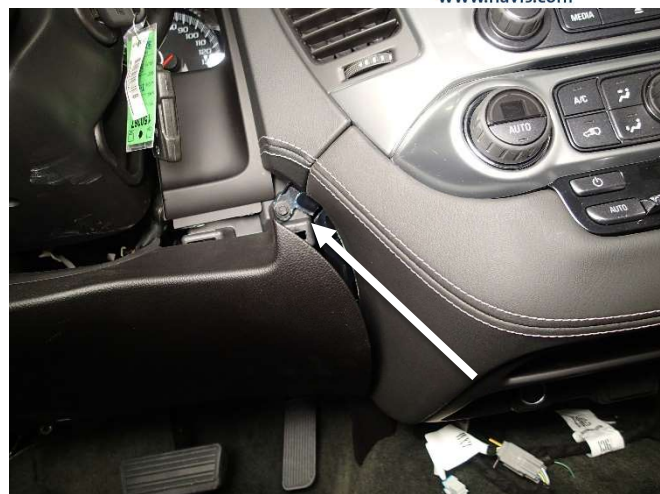
Pull back the driver side lower dash panel to gain access and remove side trim screw (7mm socket)
