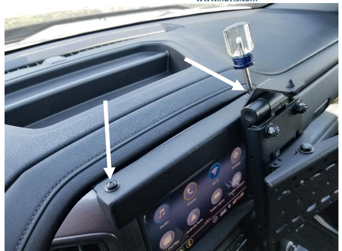
Attach the DMM-3007 frame to the upper mounting brackets first using 10-32 x 1/2" screws and #10 flat washers.
