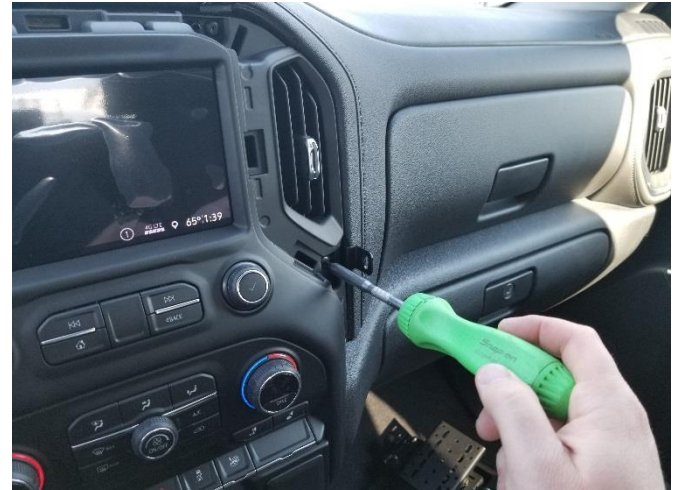
Snap trim back in and reinstall previously removed OEM screws.
