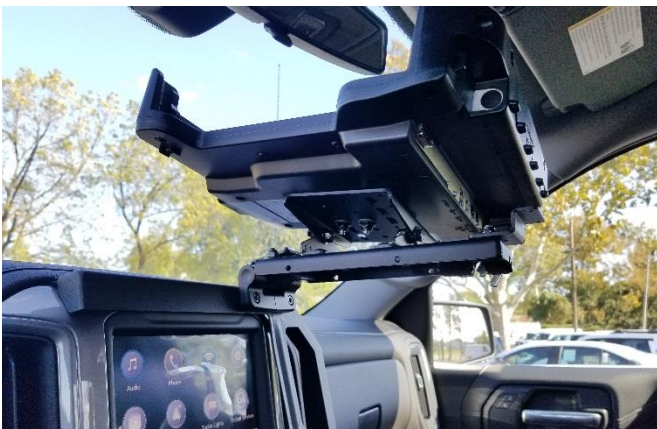
Determine desired position for your specific computer and attach to DMM swivel plate using 1/4"x 3/4" carriage bolts, PVC spacer, nylon washers, steel washers, and nylock nuts. Tighten so that the dock rotates smoothly. Tighten so dock is snug, but rotates smoothly.
