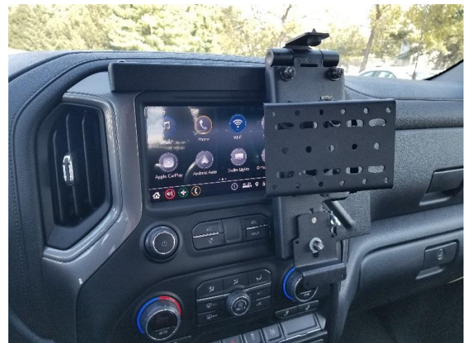
Confirm frame is tight to the dash and moves freely up and down.
