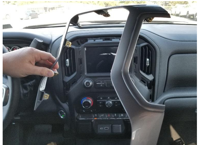
Remove trim around radio display and vents.
