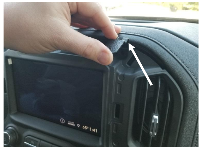
Unclip dash just enough to slide the upper mounting brackets behind the trim.
