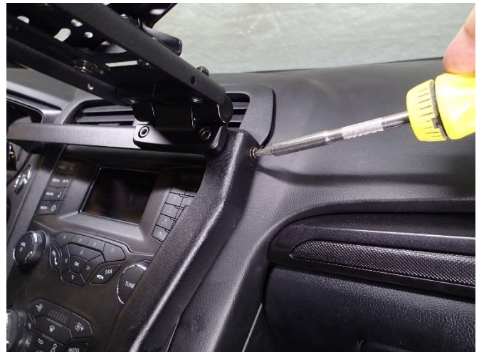
Attach frame to upper passenger side support bracket with 10-32 x 1/2" screw and star washer. (Phillips screwdriver)
