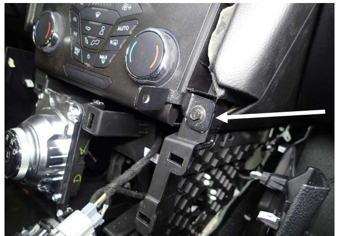
Attach passenger side lower support bracket to dash using OEM lower radio mount screw. (7mm socket)
