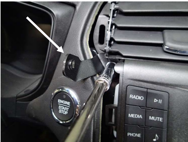
Attach driver side upper support bracket using OEM upper radio mount screw. (7mm socket)
