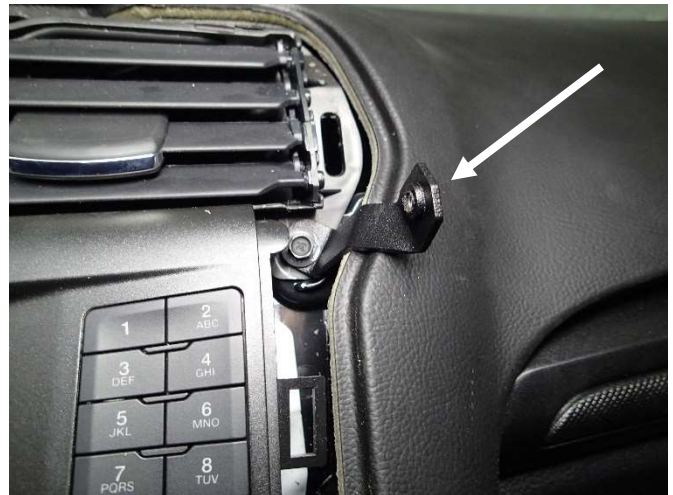
Attach passenger side upper support bracket using OEM upper radio mount screw. (7mm socket)
