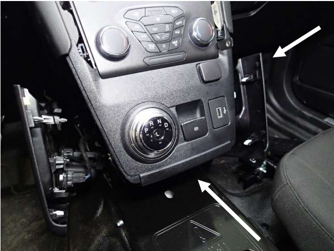
Reattach lower center and side trim panels.
