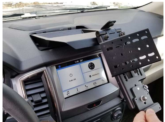
Place frame / tray and hinge mount assembly on to dash tray opening and align mount holes with top clamp bracket holes.
