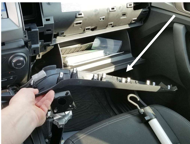
Carefully unsnap and remove lower dash trim.
