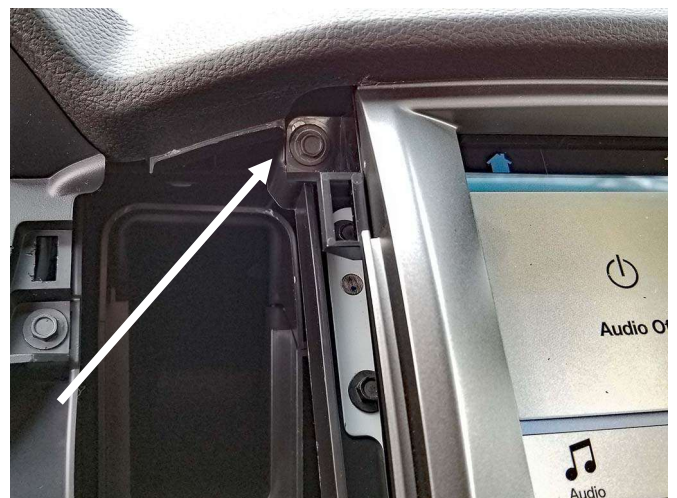
Temporarily remove upper driver side OEM display mount screw (7mm socket)
