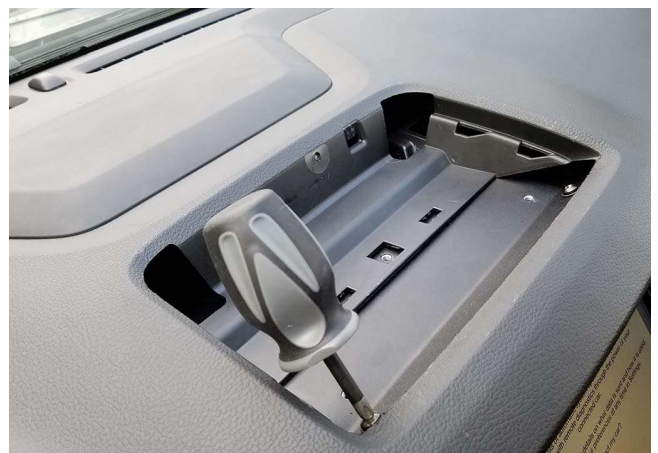
Attach the top clamp bracket to upper mount brackets with 10-32 x 1/2" Phillips machine screws and #10 flat washers.
