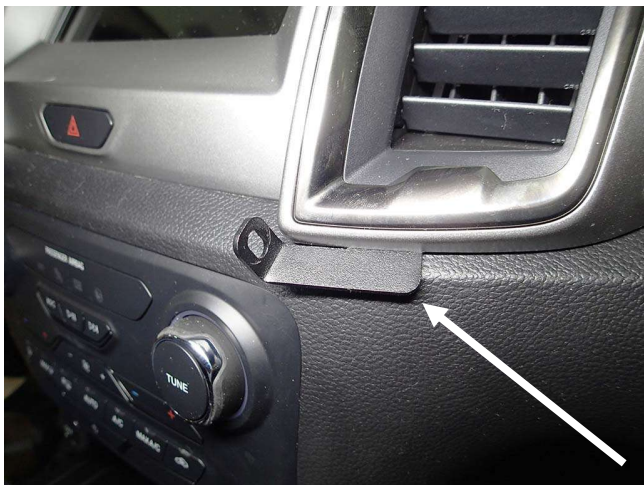
View of passenger side lower mount bracket coming out through small gap underneath vent trim.
