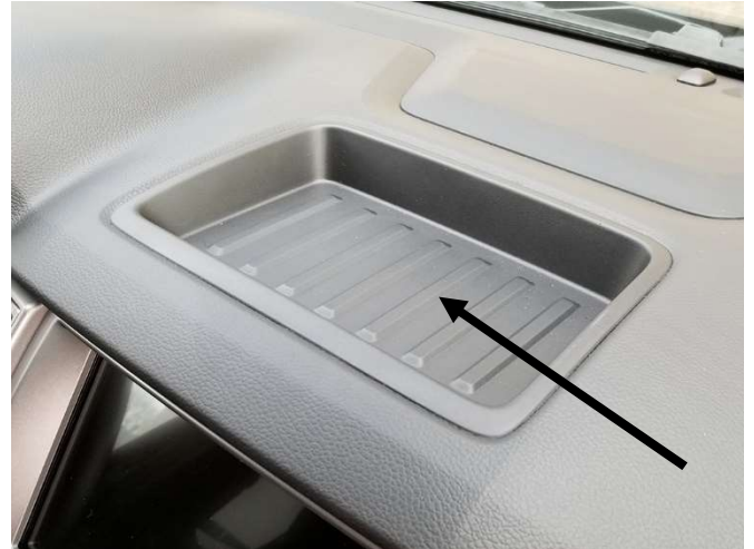
Carefully unsnap and remove the center top dash tray with panel removal tool.
