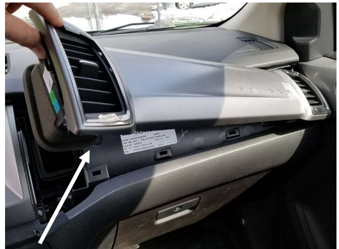
Carefully unsnap and remove passenger side vent and trim assembly.
