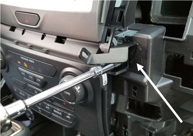
Remove lower passenger side OEM display mount screw and attach passenger side lower mount bracket with OEM screw. (7mm socket)
