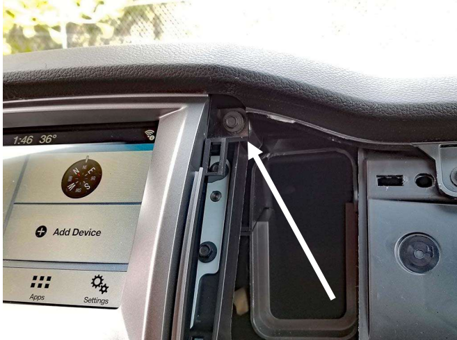
Temporarily remove upper passenger side OEM display mount screw (7mm socket)
