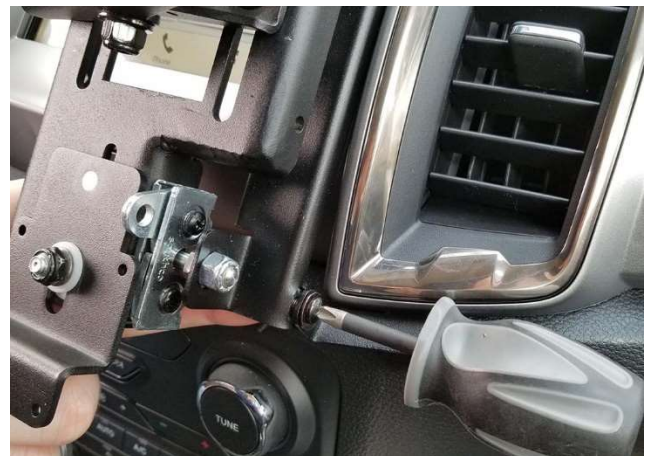
Attach frame / tray assembly to lower bracket with 10-32 x 1/2" Phillips machine screw #10 flat washer and 10-32 nut. Nut goes on the inside of frame.
