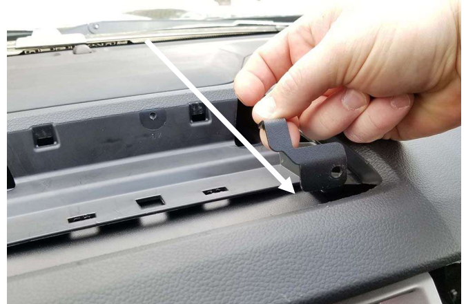
Slide passenger side upper mount bracket ( end with no threaded hole ) down from tray opening and position bracket behind passenger side OEM display mount. Do the same for driver side.
