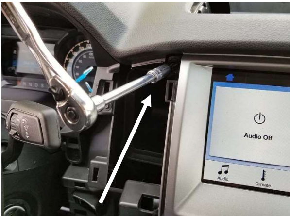
Reattach OEM display and upper brackets with previously removed OEM mount screws. (7mm socket)
