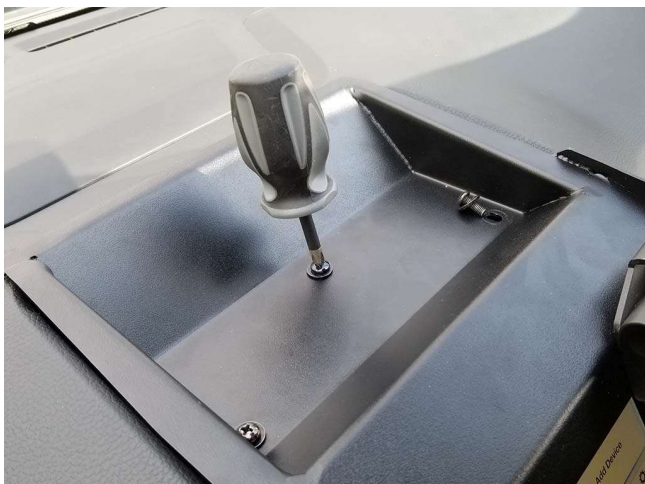
Attach frame / tray assembly to top clamp bracket with 10-32 x 1/2" Phillips machine screws and #10 flat washers.
