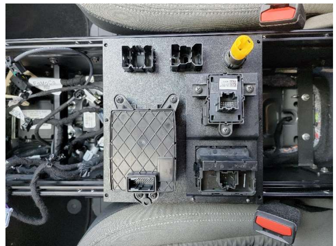
Install remaining USB and 12v sockets into shifter plate.
