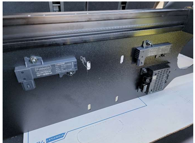
Install USB module and both key sense modules on inside of Havis console using supplied 10-32 x 1/2" machine screws and keps nuts.
