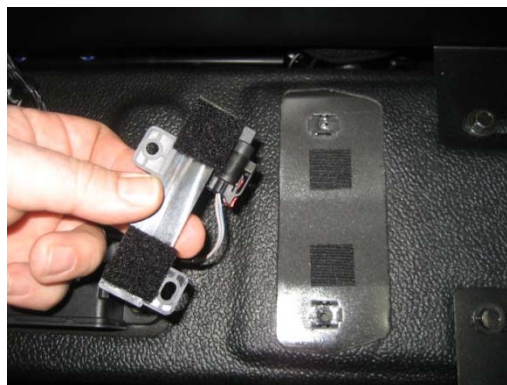
On 2011 Charger, attach Ignition proximity sensor /antenna to transmission hump with Velcro.
