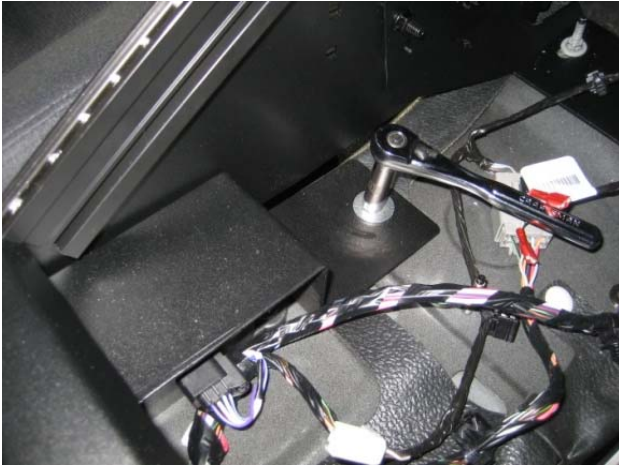
A cover is provided to guard the O.E.M. Sensor on transmission hump. If desired, attach to existing stud and 6mm nut and washer provided.
