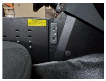
After connecting the aux panel wiring, snap panel into side trim panel.
