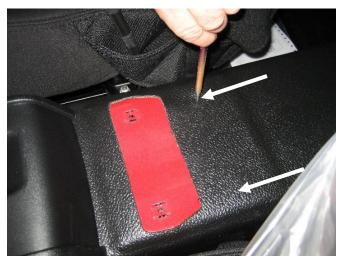
Locate inserts located under rubber mat as shown.
