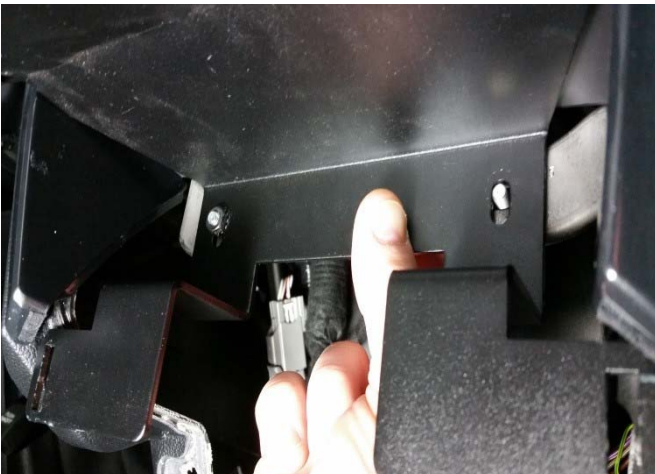
Attach console upper front support bracket to backing plate studs with 10-32 nuts
