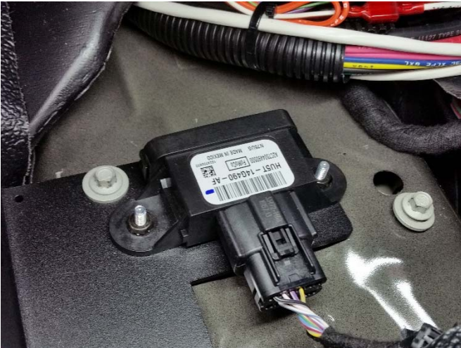
Attach restraint control module to driver mounting bracket using 10-32 keps nuts.
