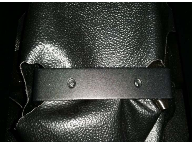
Attach rear lower bracket to existing OEM mounting flanges with supplied 6mm x 20mm hex bolts and flat washers.
