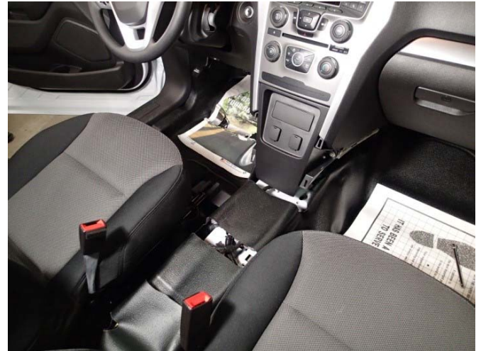
Remove OEM tunnel plate and lower dash trim included with Standard Interceptor Utility or center console included with Optional Interior upgrade.
