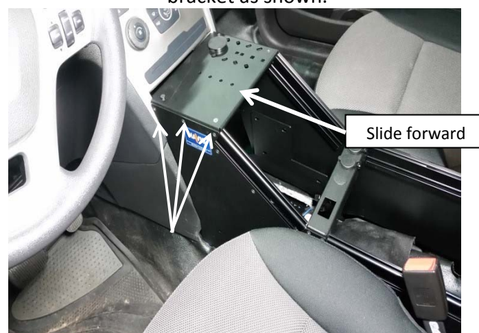
Slide console onto upper front support bracket from rear towards dash. The bracket must be above the side screws for proper alignment. Be careful not to scratch dash trim bezels
