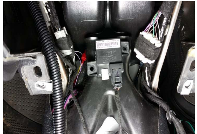
Install TPMS module onto vent with supplied Velcro.
