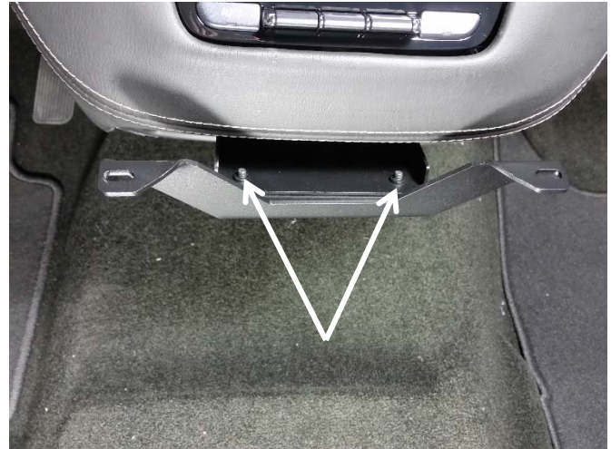
Attach the lower dash support extension (CM008737) to the bracket using 10-32x1/2" screws and washers.
