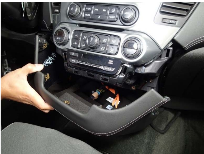
Pull lower dash panel towards you to remove. Disconnect power plugs.
