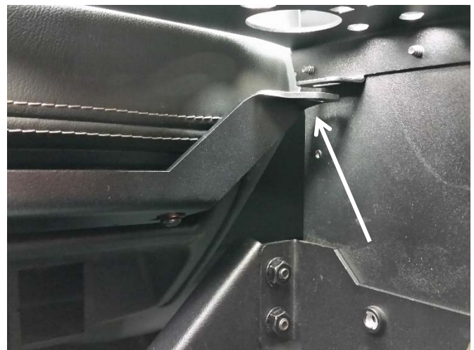
Attach console to lower dash bracket extension using 10-32 x 1/2" screws, washers, and keps nuts.
