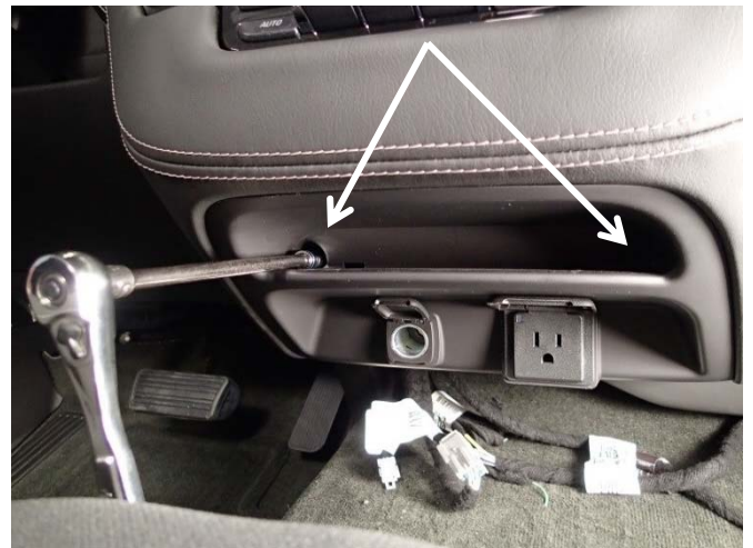
Remove rubber cover to gain access and remove two (2) lower dash panel screws. (7mm socket)
