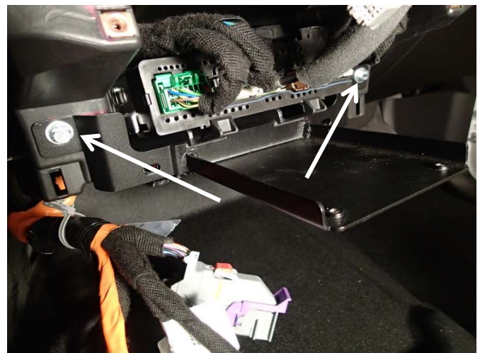
Attach Lower Support Bracket (CM006725) to existing OEM threaded holes using two (2) M6 x1.0 x 20mm bolts.
