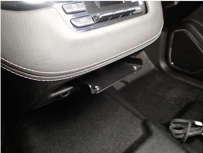
Re-install the lower dash panels and all hardware.
