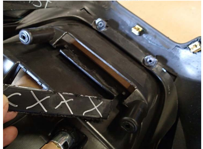
Once you've made your cut, clean and deburr the edges for a finished look.
