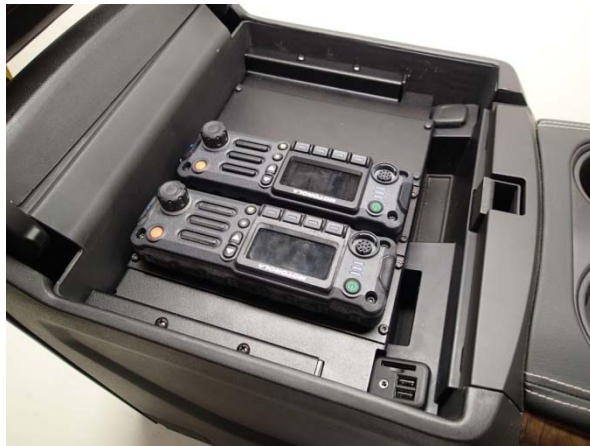
Run and connect wiring as needed and tighten all mount screws. View from passenger side
