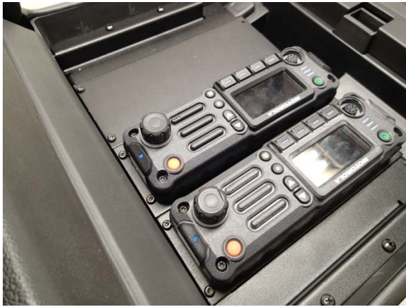
Place bezel and bracket assembly into OEM console to confirm fitment.
