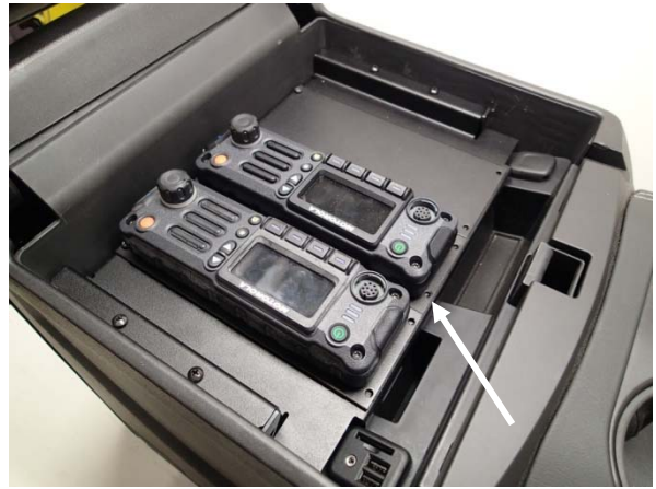
Remove assembly one more time and drill forward holes for control head brackets. Mount with # 8 x 3/8 Torx screws.
