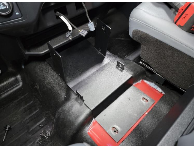
Place base mounting bracket in vehicle and line up to holes in floor.
