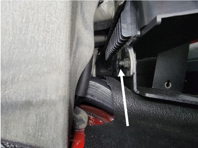
Install 1/4" serrated nuts onto the previously installed carriage bolts and tighten.
