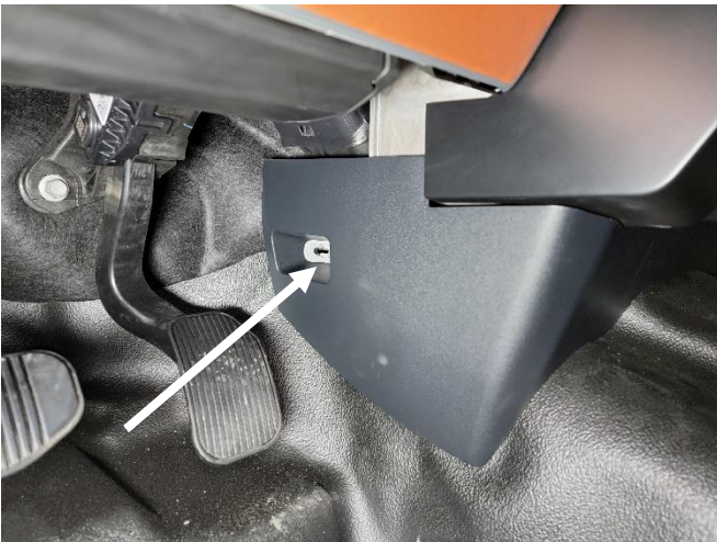
Locate 7mm head bolt from lower center of dash.
