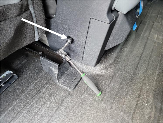
Remove bolts from rear, sides of middle seat.
