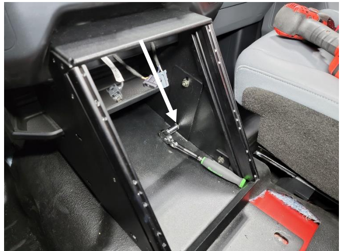
Slide console in over main mounting bracket and install using (6) 1/4" x 3/4" carriage bolts and serrated nuts.
