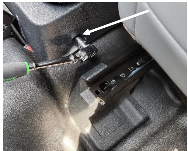
Remove bolts from front, sides of middle seat
