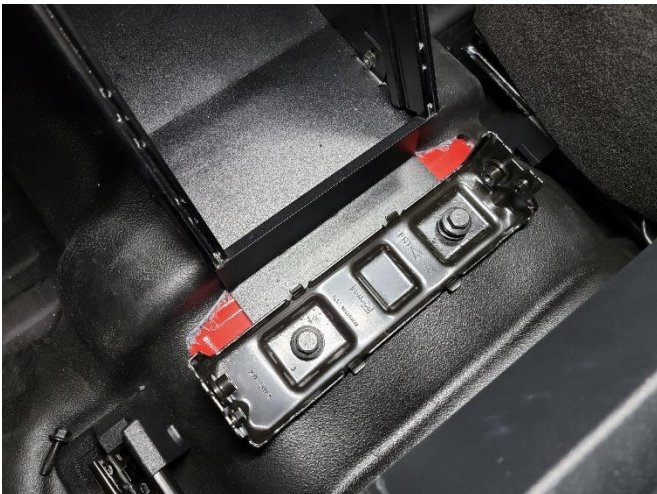
Reinstall previously removed OEM floor mounting bracket and torque to manufacturer's specifications.
