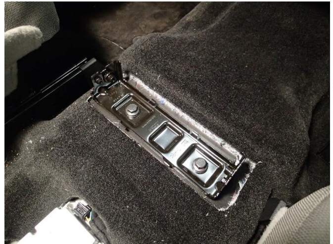
Unbolt forward, floor-mounting bracket
