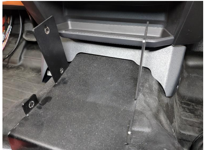
Place the lower dash trim into place, mark around mounting base and trim as needed to reinstall.
