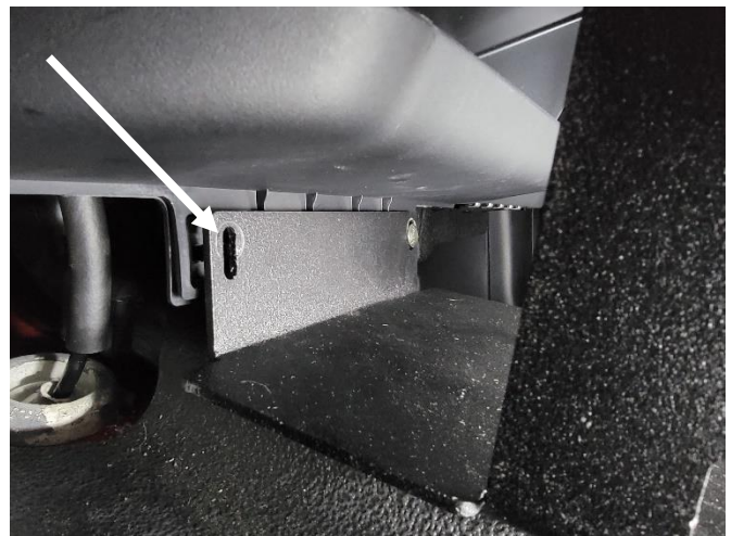
Install (2) 1/4" x 1/2" carriage bolts through the front of the bracket through the lower dash slots.
