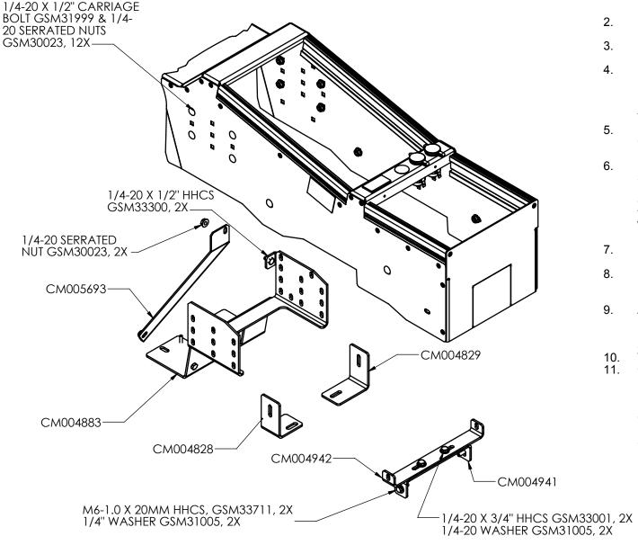
**NOTE:** 2017 INUT INCLUDES A NEW SENSOR ON THE FLOOR. FRONT BRACKET # CM004883 MANUFACTURED AFTER 11/1/16 INCLUDES STUDS AND NUTS FOR MOUNTING THE SENSOR. IF YOU HAVE AN OLDER CONSOLE, THE INSTALLER WILL NEED TO DRILL FLOOR AND PROVIDE HARDWARE FOR MOUNTING SENSOR.
