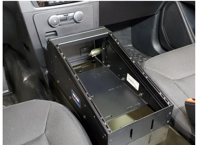
Place console on OEM tunnel plate. Slide tight to the dash.
