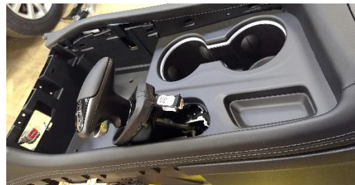
Carefully pop up shifter boot and unplug sensor from rear of boot. Loose Allen head bolt and remove shifter handle from stalk. (3.5mm)
