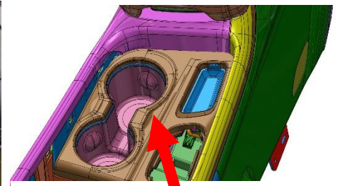
Carefully pop up the main plate OEM plate housing the cup holder and coin pocket. Unplug cup holder wires.
