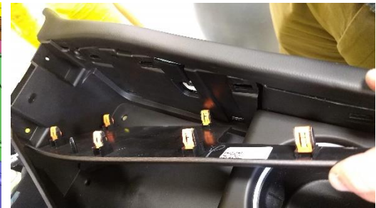
Unclip OEM front plastic sides. Remove two (2) OEM screws that hold the console down. (10mm socket) Screws to be reused.
