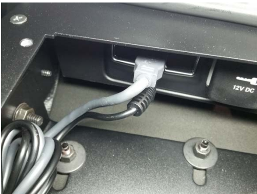
Plug in the angled USB (not shown) and aux extension wires from the Aux pass through module into the OEM aux panel on the HVAC module. Tuck wires to the side and re-install accessory pocket.
