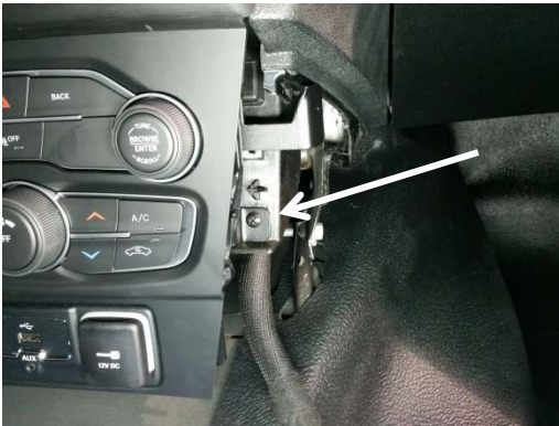
Re-install bracket and control in dash using two (2) supplied #10 X 3/4" sheet metal screws.
