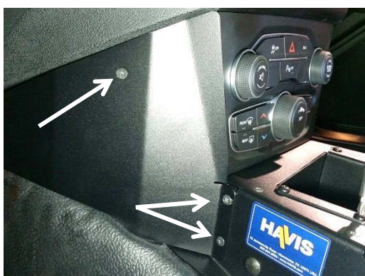
Attach driver side filler to the console and the HVAC support bracket using three (3) supplied #8 x 1/4" flat head screws. Repeat process for other side
