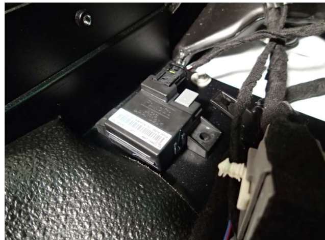
Mount sensor inside console as desired. (for 2013 -2015 vehicles only)
