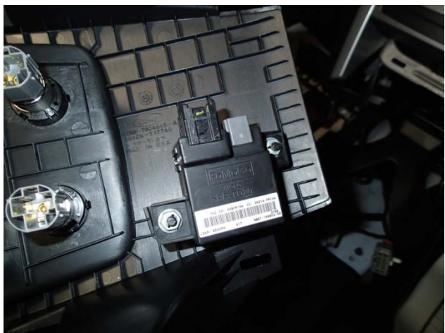
Remove sensor from back of center lower dash trim.
