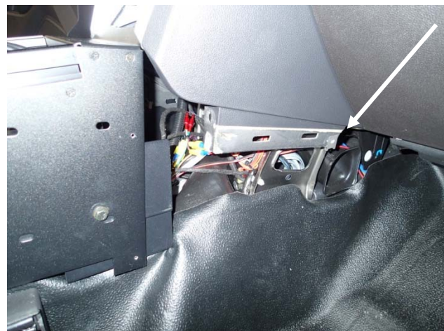
Remove side trim panel and place supplied speed nut onto drilled location. This provides a sturdy mount for trim panel screw. (follow same procedure on both sides)
