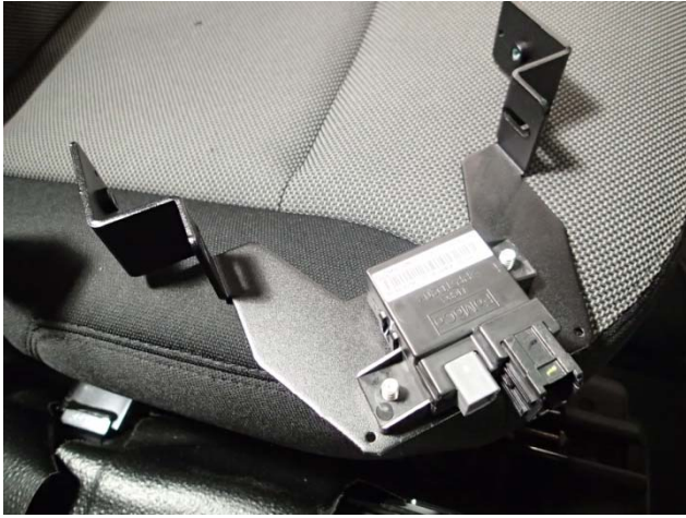
Sensor can be mounted on the underside of the rear mount bracket for the Interior upgrade 65U.
