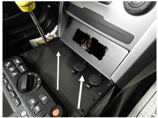
Attach top forward panel to console with 8 x 3/8" Torx screws. Install 12 volt sockets and wiring.
