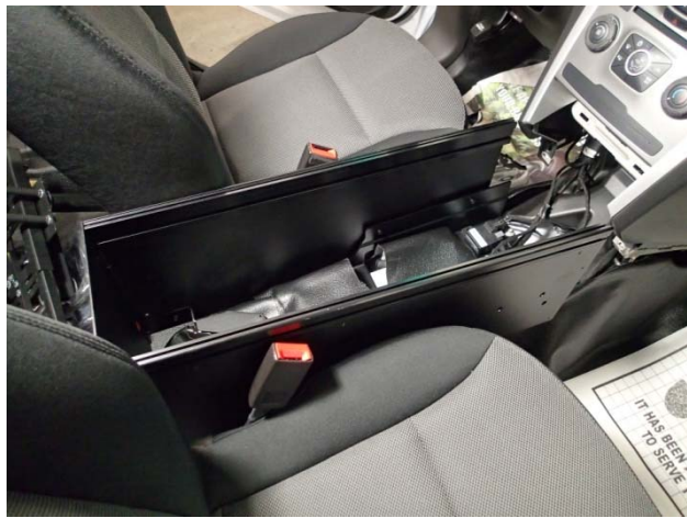
Place console housing between seats and attach sides to floor brackets with 1/4" x 3/4" Hex bolts and flat washers. (three each side)
