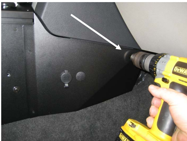
Temporarily attach side trim to console with 8 x 3/8" Torx screws and drill 1/8" hole into plastic dash panel located behind forward hole.
