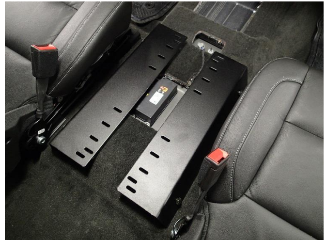
Install CM006193 hump brackets to existing OEM mount points. Use 10mm x 45mm bolts and 3/8" flat washers (Retail Tahoe) Or 3/8" x 1.75" self-threading bolts and washers for (Police Package) Between bracket and hump, use 1/2" spacers at rear and 3/4" spacers at front.
