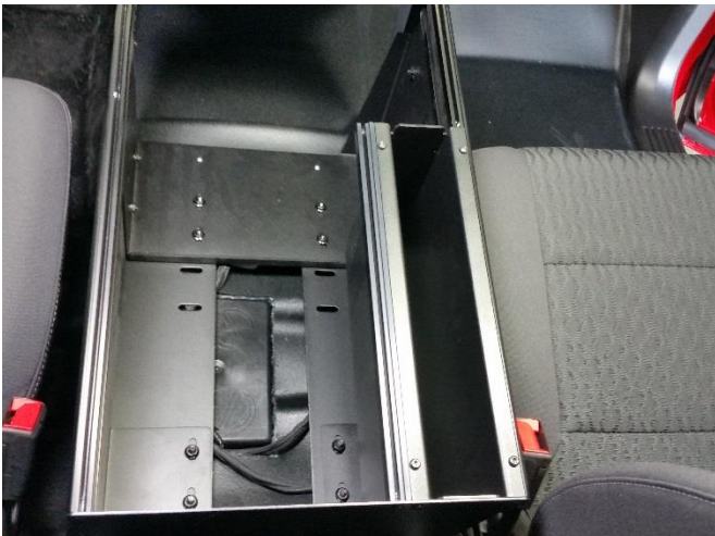
Re-install accessory pocket into the console.
