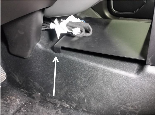
Slide the electrical accessory mounting plate (CM005915) in through the side and into place. (forward mount tabs face down)
