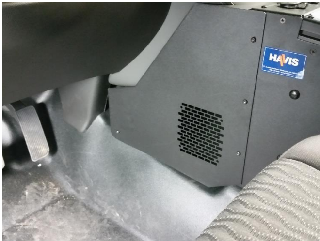
Attach driver side trim panel to console with four (4) #8 x 3/8 Torx head sheet metal screws.
