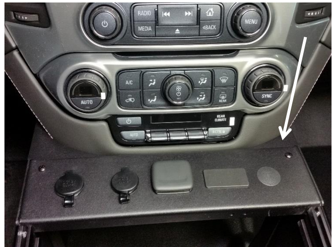
Loosely attach top trim panel (CM006409) to the underside of the console housing with 8/32 x 1/2" machine screws and Keps nuts. Install OEM aux panel.
