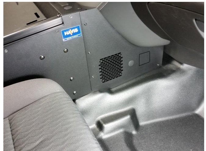
Attach passenger side trim panel to console with four (4) #8 x 3/8 Torx head sheet metal screws.
