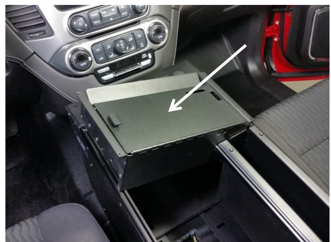
Re-install printer mount back into console.
