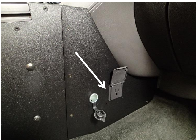
Install 12 volt and OEM 120 volt sockets in side panel if desired. Note: This photo shows the OEM 120 volt socket mounted in the side trim. OEM wire ties and tape may need to be cut in order to have enough wire to extend to this location. Splicing four (4) wire extensions may also be required. Wire and eight (8) butt connectors for extensions must be supplied by the installer.
