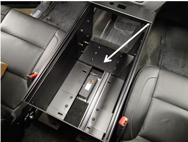
For ease of installation, remove the printer mount and accessory pocket from the console.
