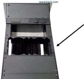
Determine 4" mounting space for cup holder and first place EB frame into console.
