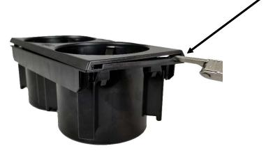
Separate the EB console mounting frame from face plate / cup holder assembly by simply inserting flat blade tool into end slots and turning.
