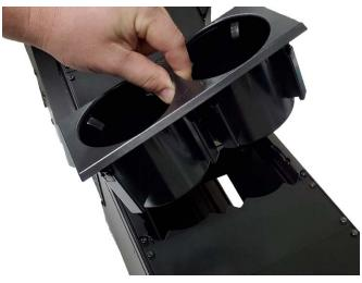
To install cup holder, pinch holder in the middle and place into EB frame until it clips.
