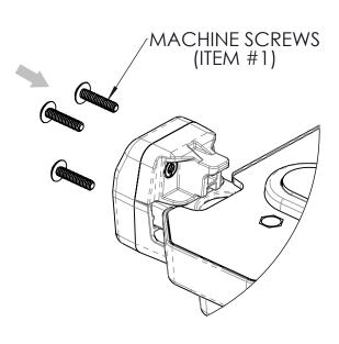
STEP 3: Attach with Machine Screws as shown, and torque to 8 in-lbs  $\pm 10\%$ . Do not over tighten, as damage can occur.
