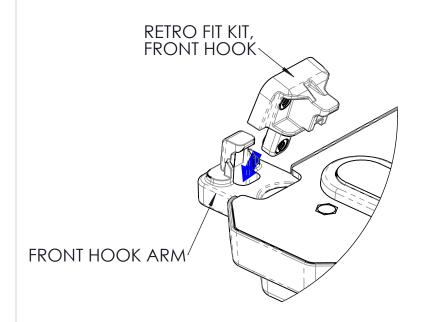
STEP 1: With the Front Hook Arms on the Docking Station extended, insert the Retro Fit Kit Front Hook into the opening of the Front Hook Arm as shown.
