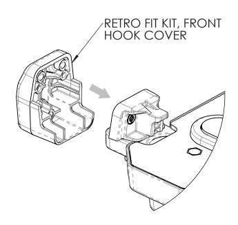
STEP 2: With the Retro Fit Kit Front Hook in place, attach the Retro Fit Kit Front Hook Cover as shown.
