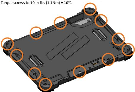
8. To remove your Apple iPad from the Havis Protective Case, simply remove the twelve screws, turn the case over, and lift the Front piece of Protective Case off the Back piece. Unplug the connector, and remove tablet.
