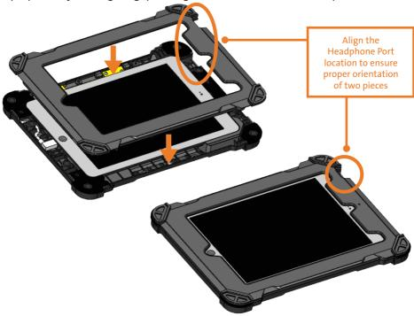
6. Holding the two pieces together, carefully turn the Protective Case over.
