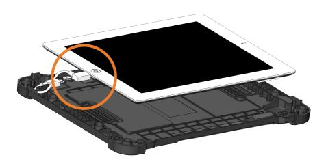
3. Place the iPad into the Back piece of Protective Case, ensuring the connector cable is routed as shown.
