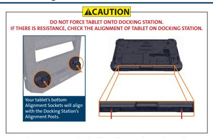
1) Ensure Docking Station is unlatched by pulling up the Latch Handles.
