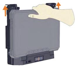
3) Once unlatched grab both sides of tablet and carefully lift up and out of the Docking Station, top end first.
