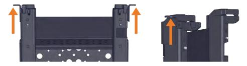
2) Hold tablet in landscape orientation, with bottom angled toward Docking Station. Lower tablet into the bottom of the Docking Station by aligning the tablet Alignment Sockets with the Docking Station's Alignment Posts.
