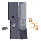
2) While holding tablet with one hand, lift the Latch Handles up and the Front Hooks will release the tablet.
