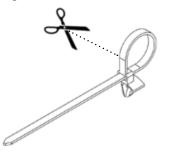
2). Pull the cut Zip Tie through the Push Pin housing. Trim excess so sharp edge does not damage reinstalled cables.
