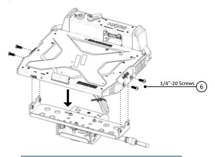
**NOTE:** It is recommended to use a drop of medium strength (blue) thread locking adhesive applied to the threads of all fasteners.
