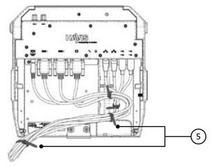
Lower the Docking Station onto the Mounting Bracket as shown, being cautious not to pinch the cable bundle. Secure with (4) 1/4"-20 screws (supplied). Torque screws to 13.4 Nm (120 in-lbs) ± 10%.
