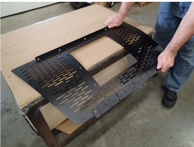
NOTE: Window guards are shipped flat. On the edge of a workbench, bend a contour in the middle of the guard so it will fit tight against the window frame.
