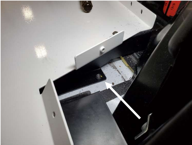
Tighten rear floor mounting hardware.
