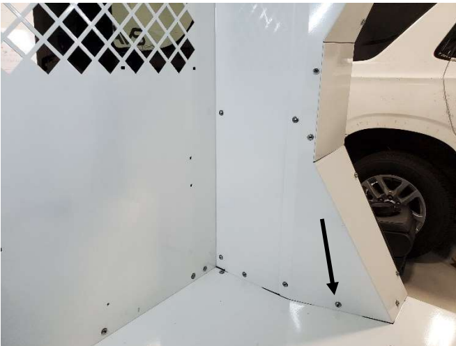
Attach to floor using 1/4" x 3/4" Phillips bolts and flat washers.
