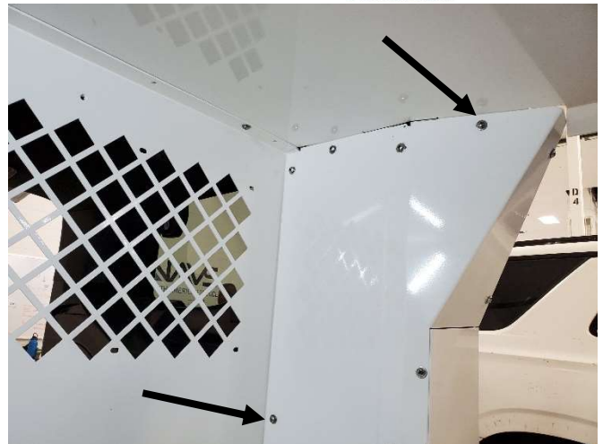
Place side filler assembly into kit and slide towards rear bulkhead. Attach to ceiling and rear bulkhead using 1/4" x 3/4" Phillips bolts and flat washers.
