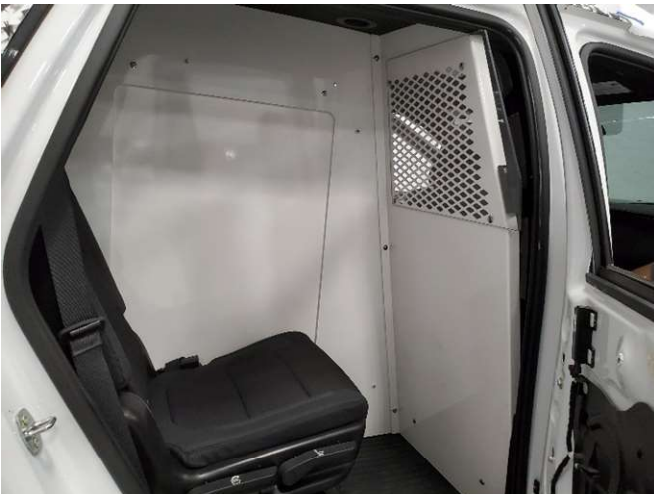
Re-install previously removed OEM seat.
