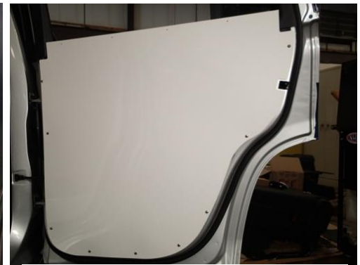
Hook door panel on the weather stripping and centering it on the door. Attach panel with # 10 x 1/2" Phillips pan head sheet metal screws.
