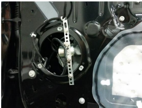
Optional door pop solenoid shown in a mounting location.
