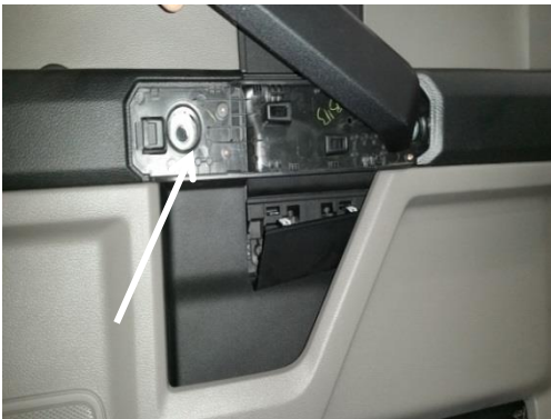
Remove two (2) bolts behind access cover behind grab handle (10mm socket)
