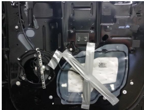
The window switch must remain plugged in proper operation. Taping the switch to the interior side of vapor barrier or wrapping in plastic bag is recommended to avoid problems with moisture.
