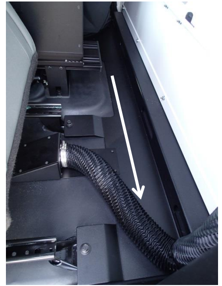
Secure the vent hose to the bottom corner of the floor bracket using supplied 15" wire tie.
