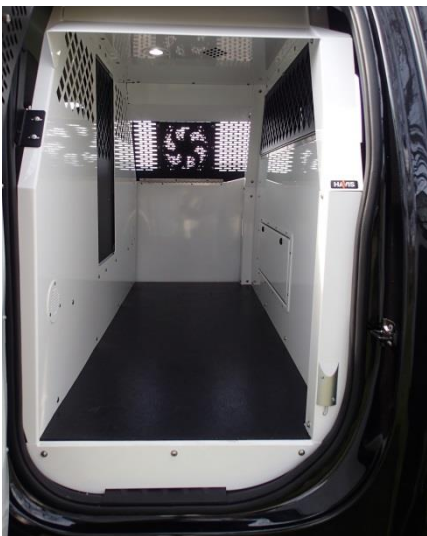
Install rubber mat. Sensor for optional NoK9 left behind feature shown.
