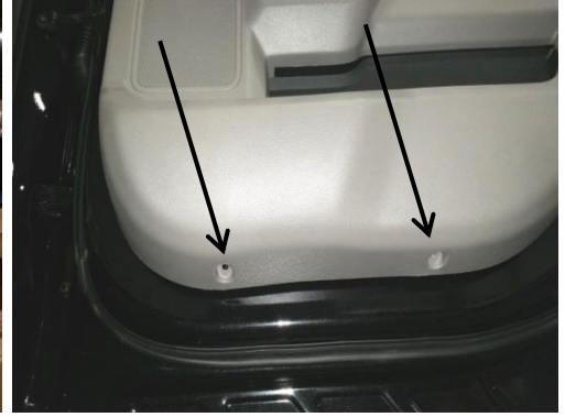
Remove two (2) screws at the bottom of the door panels (7mm socket)
