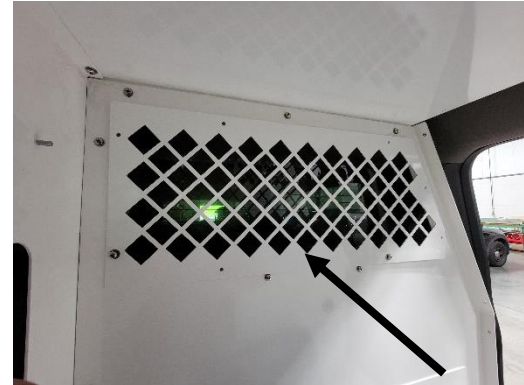
Attach rear window screen using 1/4 x 3/4 Phillips pan head bolts and washers.
