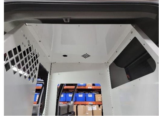
Attach the ceiling to the front and rear walls with 1/4" x 3/4" Phillips head bolts and flat washers.
