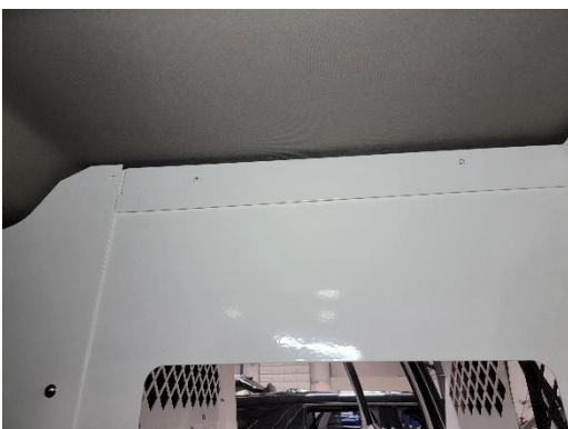
Attach upper filler panel to divider wall using 1/4" x 3/4" Phillips head bolts and flat washers.
