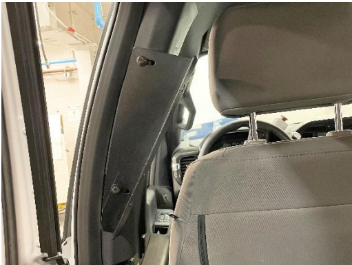
Attach outer K9 handle bracket to inner K9 handle bracket using 1/4" x 3/4" Hex head bolts and washers.
