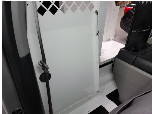
Place prisoner compartment bulkhead into truck and line up to center divider. Attach to divider using 1/4" x 3/4" carriage bolts and nuts.
