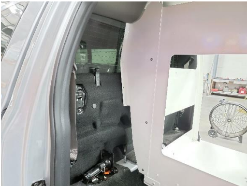
Attach side rear filler panel using 1/4" x 3/4" Phillips head bolts and flat washers.
