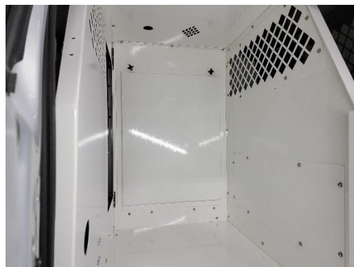
Attach emergency exit door to rear divider with two (2) knobs. Silicone floor are seams and let dry before placing in rubber floor mat.
