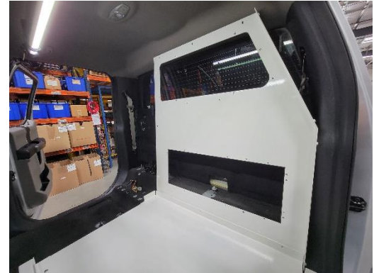
Attach rear wall and floor to the floor bracket using 1/4" x 3/4" Phillips pan head bolts and washers
