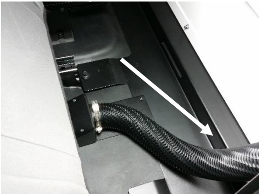
Secure the vent hose to the bottom corner of the floor bracket using supplied 15" wire tie.
