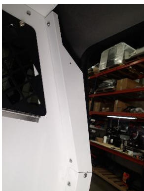
Loosely attach K9 upper side filler panel to rear wall with 1/4 x 3/4 Phillips pan head bolts and washers.
