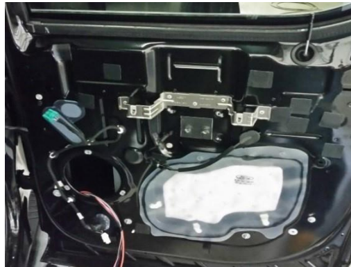
Disconnect door latch cable and lock pin. Remove speaker. (7mm socket) Remove window switch from door panel and set aside.
