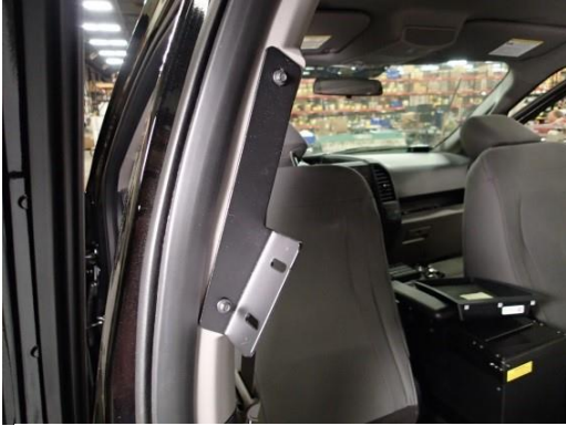
Install upper mounting bracket using previously removed M6 hardware.
