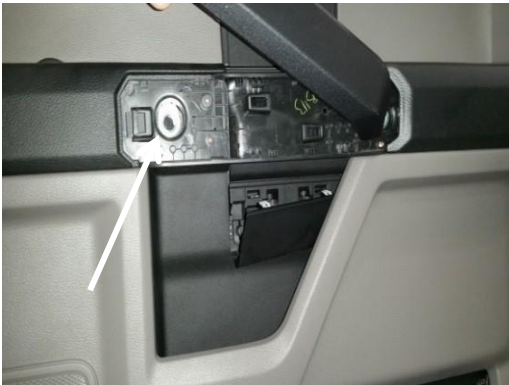
Remove two (2) bolts behind access cover located behind grab handle. (10mm socket) Carefully pull off door panel.
