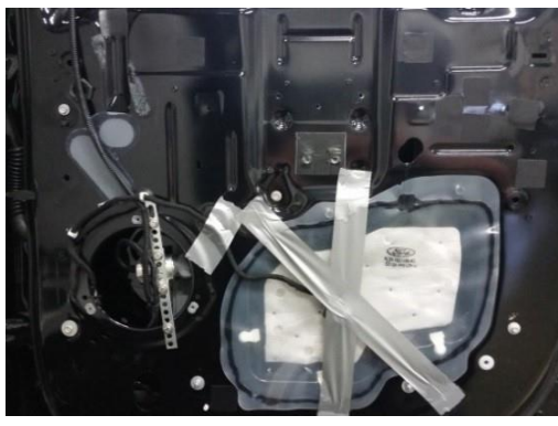
The window switch must remain plugged in for proper operation. Taping the switch to the interior side of vapor barrier or wrapping in plastic bag is recommended to avoid problems with future moisture issues.
