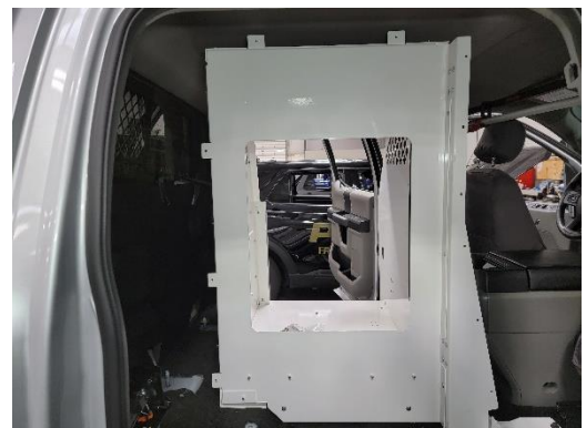
Place divider wall in truck and line up to floor and front bulkhead.
