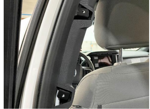
Reinstall previously removed OEM "B" pillar trim.
