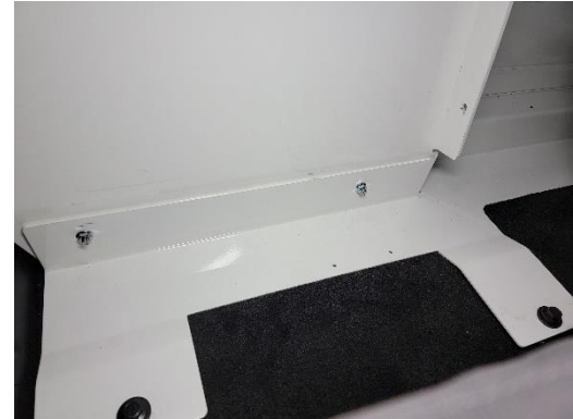
Attach bulkhead to lower floor mounting bracket using 1/4" x 3/4" carriage bolts and nuts.
