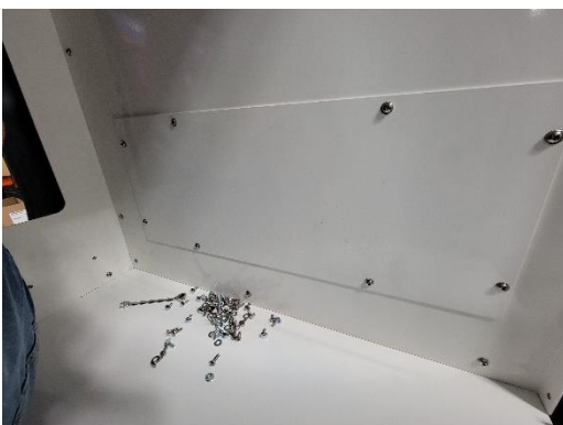
Attach lower rear access cover using 1/4 x 3/4 Phillips pan head bolts and washers.
