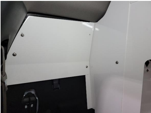
Install rear window guard between rear filler panel and C pillar bracket using 1/4" x 3/4" Phillips head bolts and flat washers.
