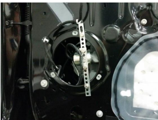
Optional door pop solenoid shown in a mounting location.
