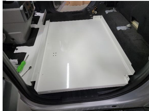
Attach floor to the front base mounting bracket using four (4) 1/4" x 3/4" carriage bolts and serrated nuts. Access to the center bolts is available through the slots in the bracket.
