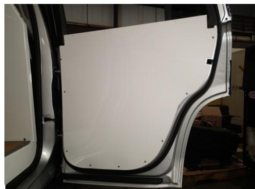
Hook new door panel on the weather stripping and centering it on the door. Attach panel with # 10 x 1/2" Phillips pan head sheet metal screws.
