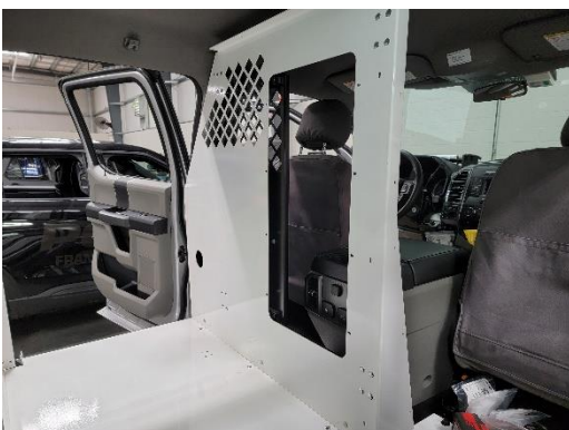
Attach front wall to "B" pillar brackets using 1/4" x 3/4" carriage bolts and serrated nuts.
