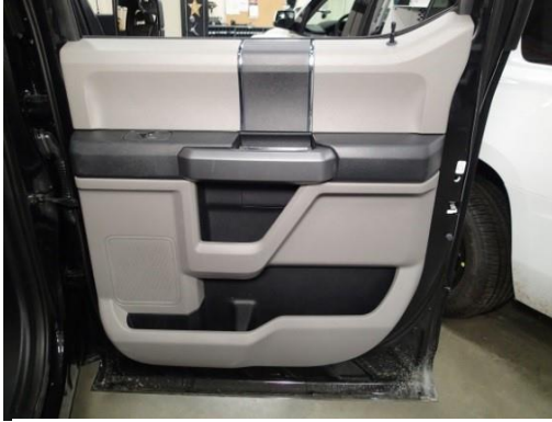
Remove rear passenger door panels first.
