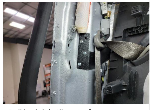
Pull back (C) pillar trim from passenger, rear of truck and line up bracket. Bracket should line up with existing hole in metal frame. Drill and attach using (3) 10 x 1/2 Phillips pan head sheet metal screws.
