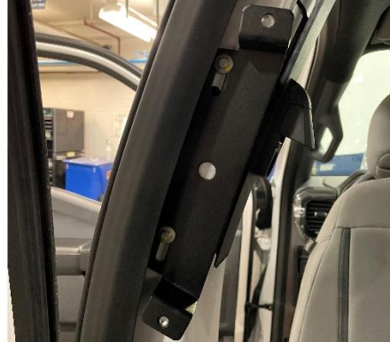
On the 2021+ F-150, remove the OEM "B" pillar trim and OEM handle. Attach inner K9 bracket to "B" pillar using previously removed OEM handle hardware.
