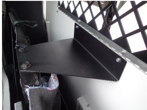
Attach the upper rear support bracket to holes in rear wall and to OEM threaded holes with previously removed seatbelt hardware.
