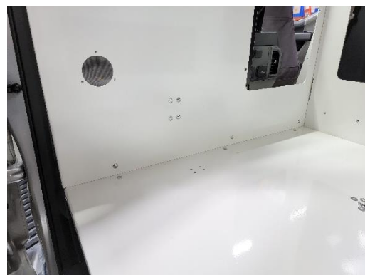
Attach front wall to floor using 1/4" x 3/4" carriage bolts and serrated nuts.
