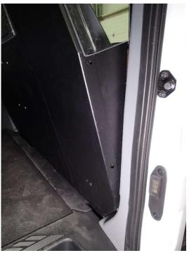
Attach lower side fillers with 1/4"x 3/4" carriage bolts, washers and nylock nuts.
