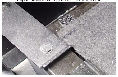
Attach front lower support brackets (CM007238) to pre-drilled holes in seat base using 1/4"x 3/4" hex bolts, 1/4" washers, and nuts. (one each side)
