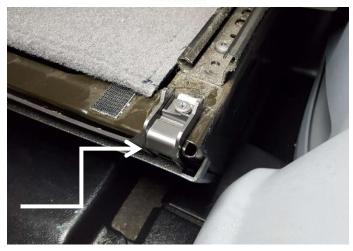
**NOTE**: If vehicle has OEM plastic clips that hold rear trim panel to these holes, clips and trim must be permanently removed.
