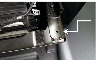
Slide front passenger seat forward and remove cover under seat. Drill out the existing outboard hole in seat base to 1/4".
