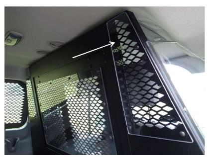
Install additional clear polycarbonate wings using 1/4"x 3/4" carriage bolts, washers, and nylock nuts.
