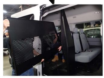
With the help of another person load the upper main panel into the van. Line up the holes to the lower base.
