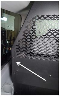
Attach the side reinforcement bracket to the upper and lower base using four (4) 1/4 x 3/4" carriage bolts and nuts.
