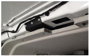
With the bracket between headliner and roof, line up to the OEM hole in rib, mark and carefully drill seven (7) 1/8" pilot holes in the rib and attach bracket using #10 x 1" screws (GSM33196)
