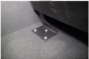
Attach driver side bracket to floor with three (3) 1/4 x 1" Lag screws. *Take caution not to strip the holes.*
