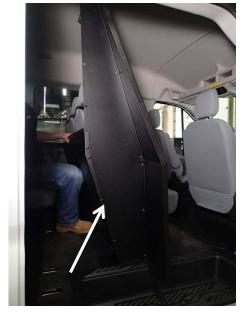
Attach side support panels to the lower partition base with four (4) 1/4 x 3/4 carriage bolts and nuts.
