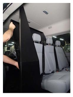
While holding the upper main panel in place lean both main panels back and install 1/4 x 1/2" carriage bolts into the holes. Have another person attach the nuts from the forward side.
