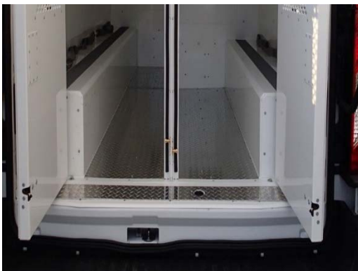
Adjust doors as needed for proper alignment to pins. Loosening of the bolts on the hinge to raise or lower the door may be necessary. The latches should meet the pins evenly and engage both stages when closing.
