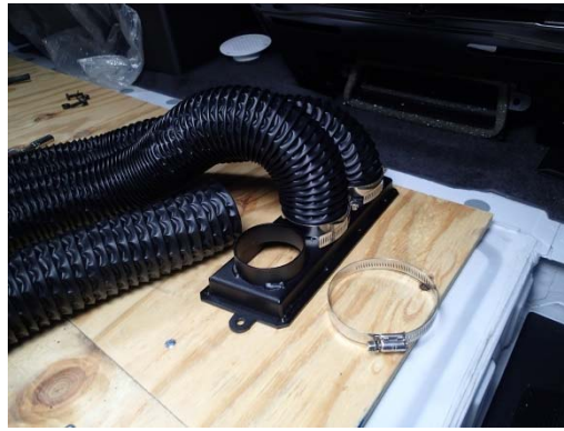
Attaching the heater hose and clamps to the front plenum assembly (KKM006916) before installing is recommended.
