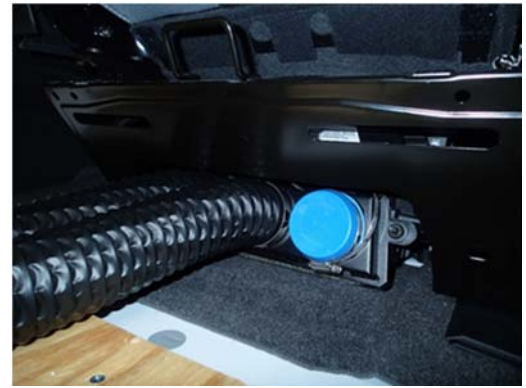
If you're not installing a 3 compartment kit then you will need to install a vent cap (PRM97503) on one of the outlets in the plenum.
