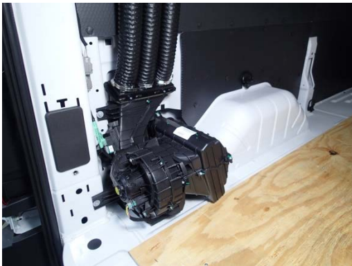
Attach the Air Conditioning hose and clamps to the plenum assembly
