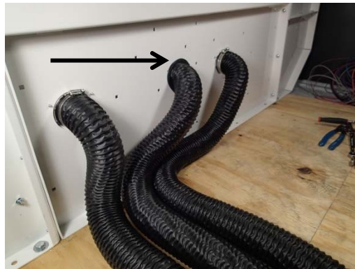
If installing a 3 compartment kit you will need to run a hose through the middle hole in the bulkhead. This will allow the hose to run underneath the bench and attach to the middle bulkhead. Run gimp around the hole in the front bulkhead before running the hose through.
