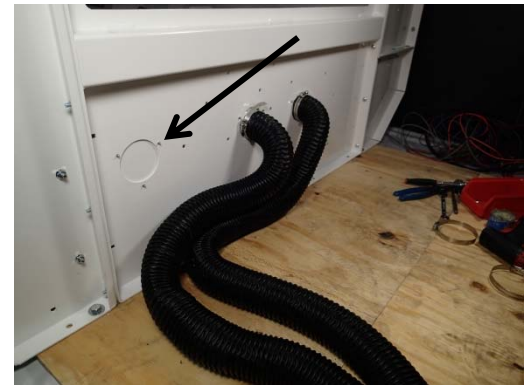
On the one and two compartment kits you will need to use the vent block off (KKM0403-004) on the opening closest to the passenger side of the kit
