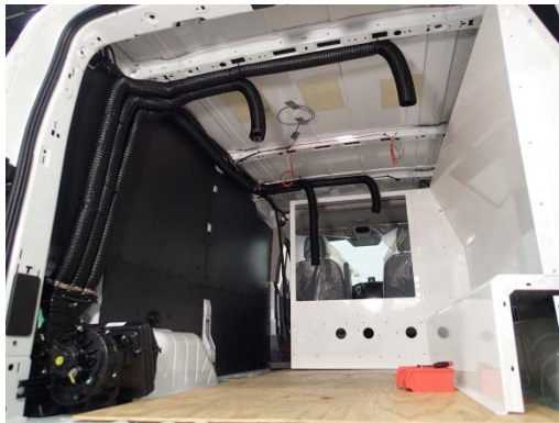
Run a single long length of hose and attach the "Y" and split the hose into two vents in driver and passenger side front ceiling. This will provide a total of four ceiling vents.
