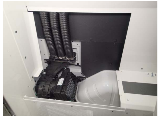
This shows the rear access panel removed and the factory AC system. This cover is easily removable for serviceability in the event of failure.
