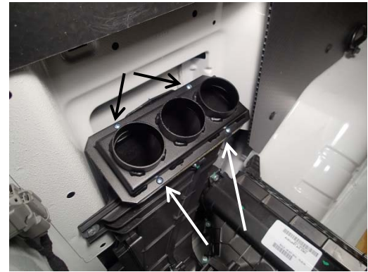
Install the vent adaptor (KNM006915) onto the blower motor of the OEM rear AC unit using four (4) #10 x 3/4" screws.
