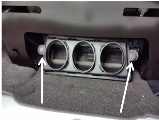
Install the plenum (KNM006916) to the blower motor using two (2) 1/4" x 3/4" bolts and 1/4" serrated nuts. (Plenum shown without hoses to show hardware)
