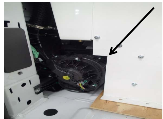
NOTE: If retrofitting a Prisoner Transport out of an older van the following modification will need to be made to the rear bulkhead to clear the factory or aftermarket blower motor assembly. Approximately 8" x 1.25" must be cut out of the left side of the bulkhead.
