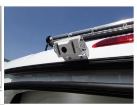
Mount external camera in desired location. If being used for viewing when backing up install camera on backside of roof as close to center as possible. The "U" shape bracket included with camera should work in most applications.
