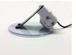
Attach camera to the Camera mounting bracket using two (2) 10-32 x 1/2" bolts and 10-32 keps nuts. Attach the bracket to the cover with two (2) 10-32 flat head screws and keps nuts.
