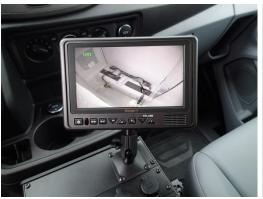
Plug camera cable into one of the camera assemblies. Turn on system. Position the camera to obtain optimal visibility within the compartment. You will need two people for this step.
