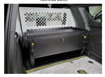
Attach the rear trim to the bottom of the SBX-1000 drawer using #10 sheet metal screws into pilot holes drilled in step 1.
