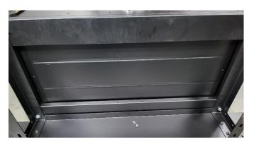
Run the screws into the pilot holes to form the threads while there is easier access to the holes. If parts were preassembled, remove the trim panel after this is complete. Risers can remain attached.
