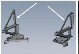
Attach side-mounting braces onto the side of upper mounting brackets using 5/16" x 1" bolts, washers, and nylock nuts.
