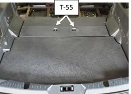
Remove both sections of the OEM trunk floor.
