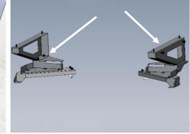
Place drawer assembly into vehicle and line up to the mounting points in the mounting base. Attach using (4) 5/16" x 1" bolts, flat washers and split lock washers.
