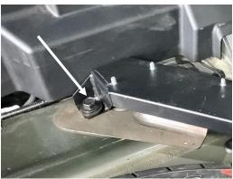
Remove rear bolt from OEM cross brace and install lower mounting bracket re-using OEM bolt. Repeat for passenger side Havis, Inc. 75 Jacksonville Road Warminster, PA 18974 T 800-524-9900 F 215-957-0729 www.havis.com
