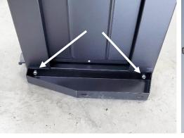
Attach upper mounting brackets to the bottom of the SBX box using (4) 5/16" x 3/4" thread forming bolts. Run bolts in and out once prior to attaching bracket to start threads
