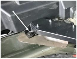
Remove rear bolt from OEM cross brace and install lower mounting bracket re-using OEM bolt.
