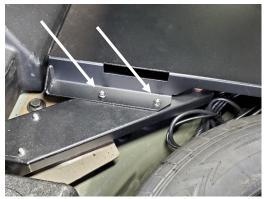
Place mounting base in the vehicle and attach to studs using (4) 1/4" serrated nuts.
