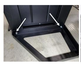
Attach upper mounting brackets to the bottom of the SBX box using (4) 5/16" x 3/4" thread forming bolts. Run bolts in and out once prior to attaching bracket to start threads.
