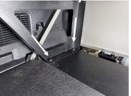
Place drawer assembly into vehicle and line up to the mounting points in the mounting base. Attach using (4) 5/16" x 1" bolts, flat washers and split lock washers.
