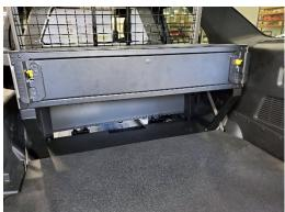
Attach block off plate to forward section of risers using (6) 10-32 x ½" screws and washers.
