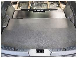
Place rear section of factory floor back in vehicle.
