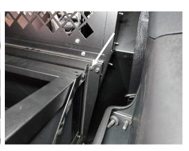
Tighten hardware at rear cross brace of K9 wall.
