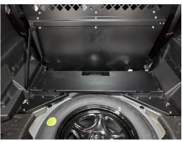
Make sure brackets are loose and pushed against the sides of the cargo area.
