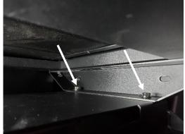
From underside of SBX box, install 5/16" x 1" bolts, split lock washers, and nuts into mounting base.
