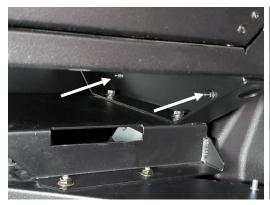
Attach side, mounting brackets to risers using 5/16" x 1" bolts, flat washers, and nylock nuts.
