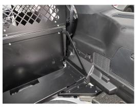
Loosely install side, mounting bracket. Attach to rear cross brace of K9 rear wall using 1/4" x 3/4" Phillips pan head bolts and washers.
