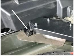
Remove rear bolt from OEM cross brace and install lower mounting bracket re-using OEM bolt.
