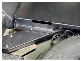
Place mounting base in the vehicle and attach to studs using (4) 1/4" serrated nuts.
