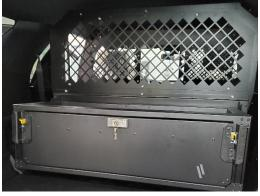
Place SBX box into back of vehicle on top of base plate and between side mounting brackets.
