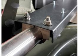
Attach other end of lower support bracket with supplied U-bolt, flat washers, lock washers and nuts.
