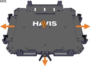
2) Place computer in center of unlatched Universal Cradle, ensuring the device is touching both Front Fences as well as the Rear Fence, then push inward on both Side Trays until a click is heard.
